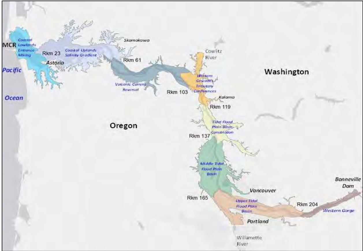
1240 1241 Figure 2-18. Lower Columbia River and Estuary Represented by Eight Hydro-Geomorphic 1242 Reaches 1243 Note: Each HG reach characterizes similar attributes of river morphology, sediment transport, and hydraulic/tidal 1244 conditions. River kilometers denote boundaries between reaches, 1 kilometer (km) = 0.62 miles. 1245 Source: Simenstad et al. 2011
