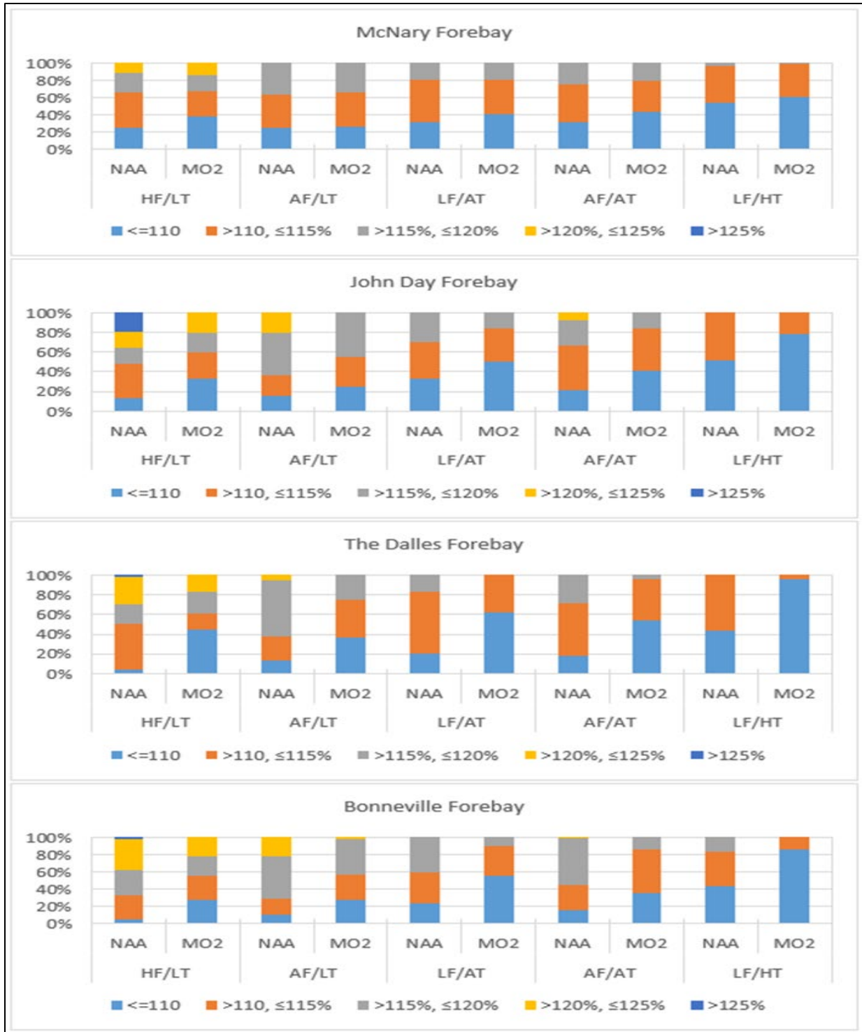
4220 4221 Figure 5-55. Frequency of modeled forebay Total Dissolved Gas violations of current 115 4222 percent Total Dissolved Gas State water quality standards during current fish passage spill 4223 season for the No Action Alternative and Multiple Objective Alternative 2 at McNary, John 4224 Day, The Dalles, and Bonneville Dams under a 5-year range of river and meteorological 4225 conditions 4226 Note: Current fish passage spill season is from April 1 to August 31.
