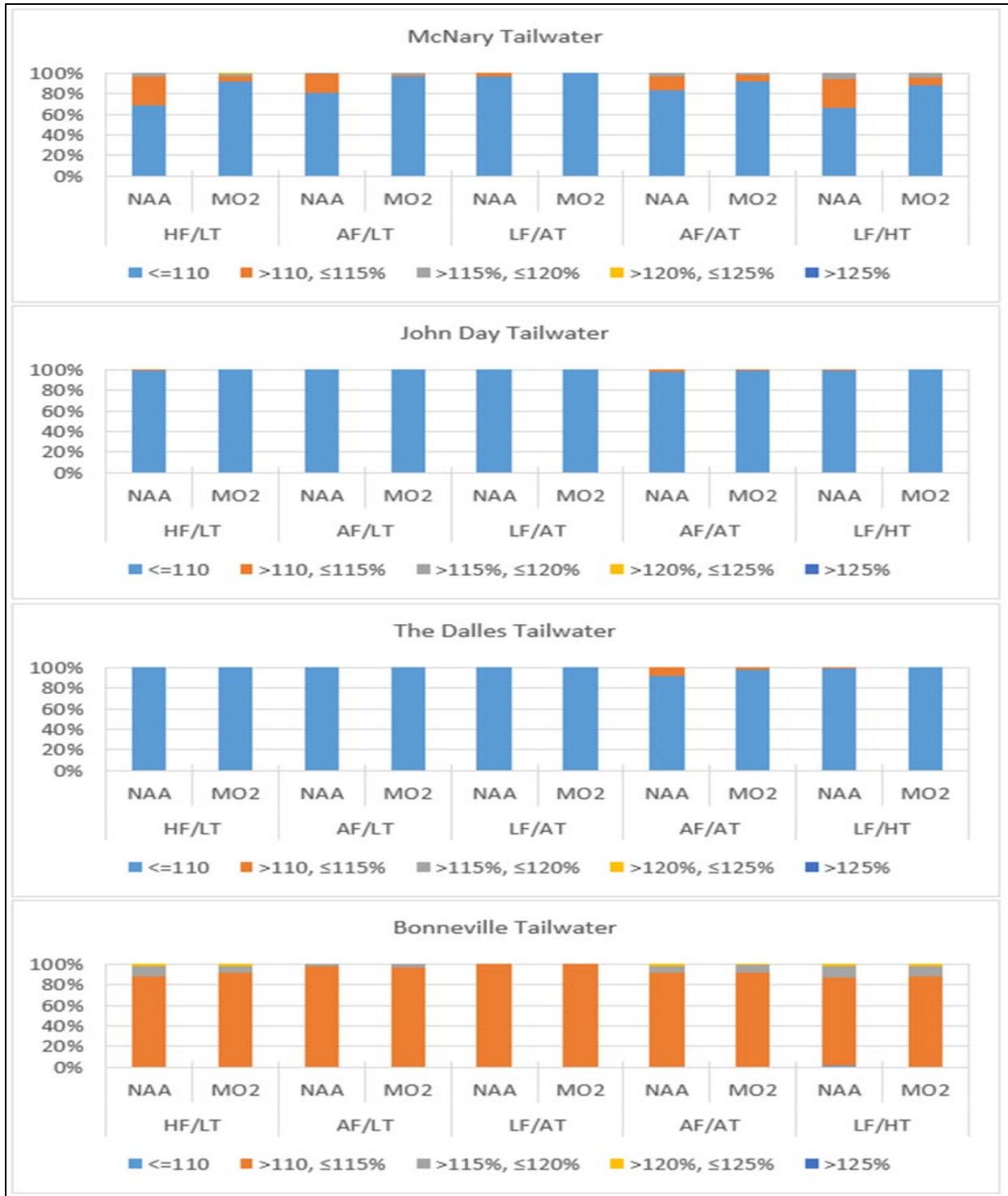
4239 4240 Figure 5-60. Frequency of Modeled Tailwater Total Dissolved Gas Outside of Current Fish 4241 Passage Spill Season for the No Action Alternative and Multiple Objective Alternative 2 at 4242 McNary, John Day, and The Dalles Dams Under a 5-Year Range of River and Meteorological 4243 Conditions
