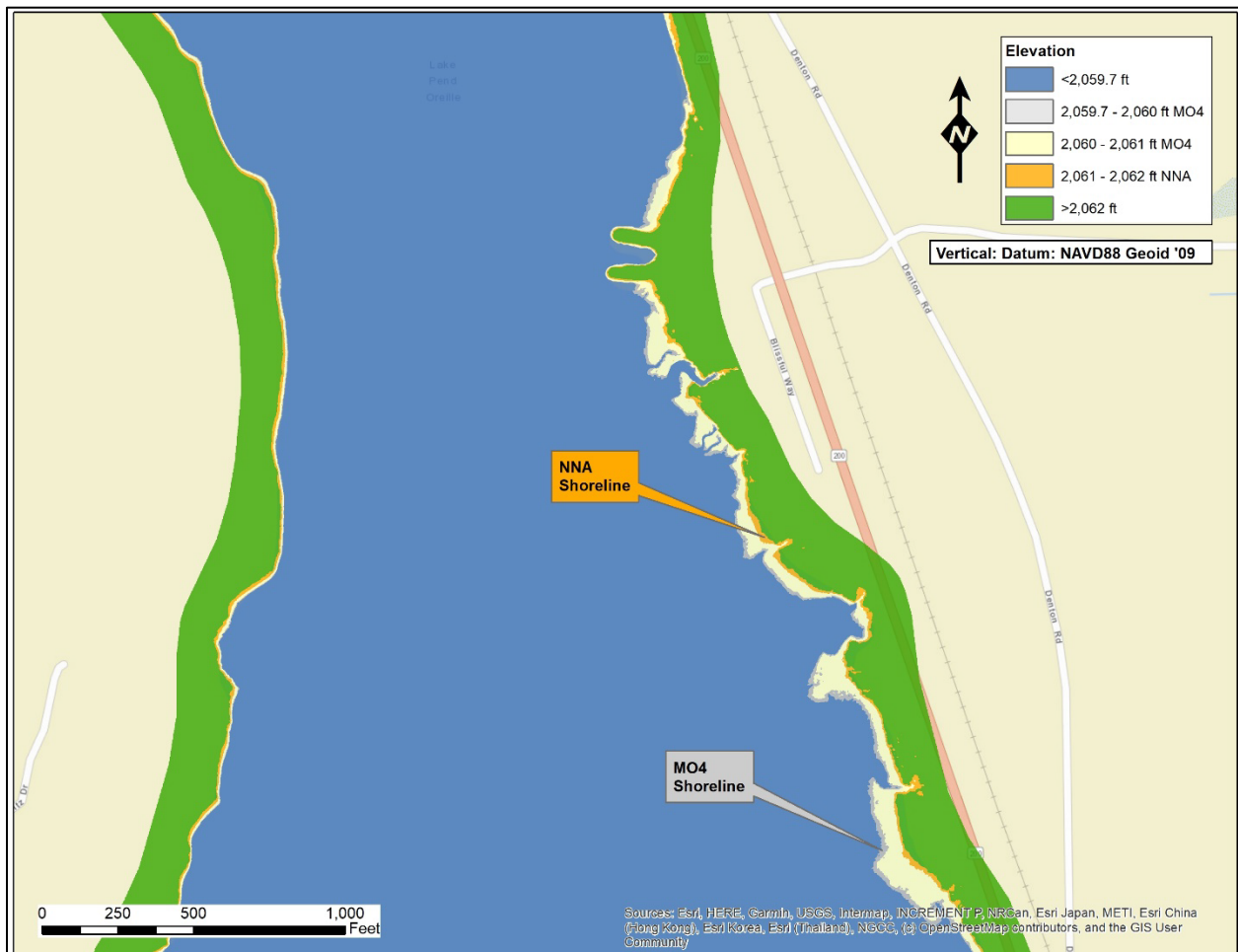
23696 Figure 3-154. Shorelines of Denton Slough in Lake Pend Oreille Showing Average Land 23697 Exposure for the No Action Alternative and MO4
