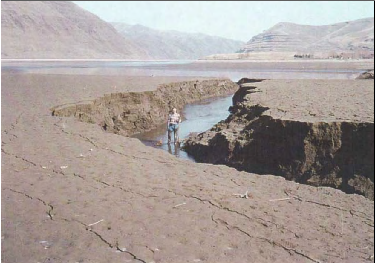
Figure 3-29. Tributary Incision Through Deposited Sediments at Alpowa Creek during the 1992 Drawdown of Lower Granite Dam
