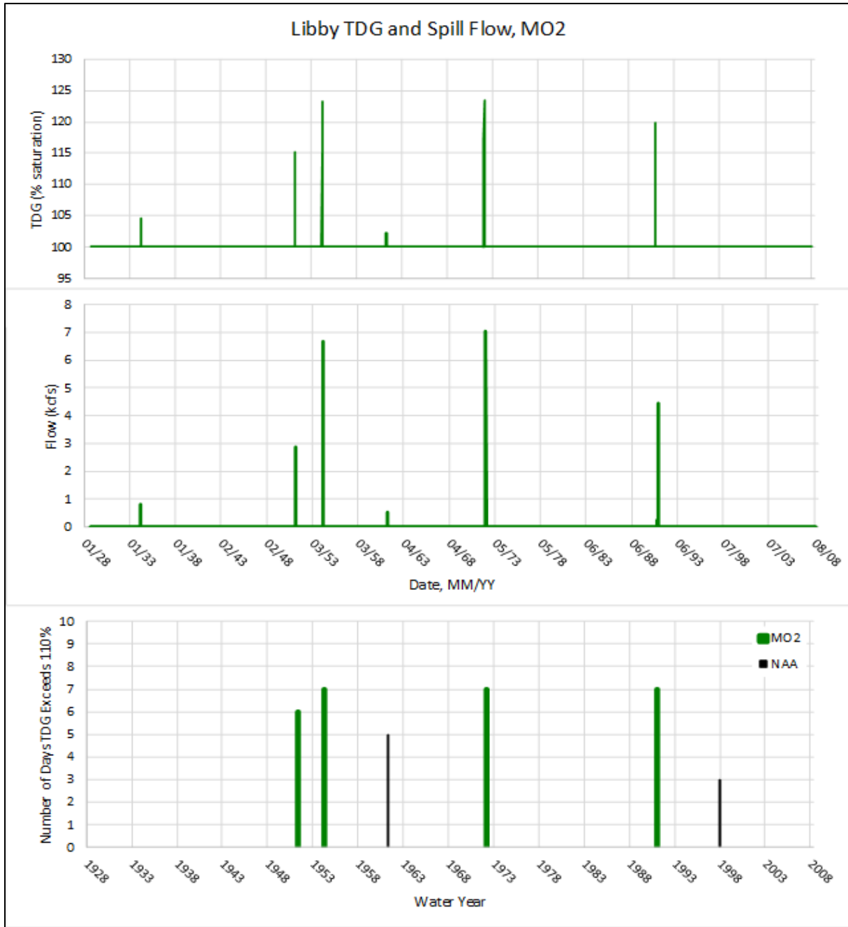
Figure 5-12. Modeled Tailwater Total Dissolved Gas and Spillway Flows for the Multiple Objective Alternative 2 and the Number of Exceedances for No Action Alternative and Multiple Objective Alternative 2 at Libby Dam over an 80Year Period
