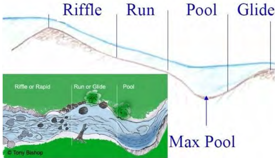
Figure 3-3. Depiction of stream habitat classifications. Riffles are fast and shallow; runs are fast and deeper; pools are slow and deep; and glides are slow and shallow.
