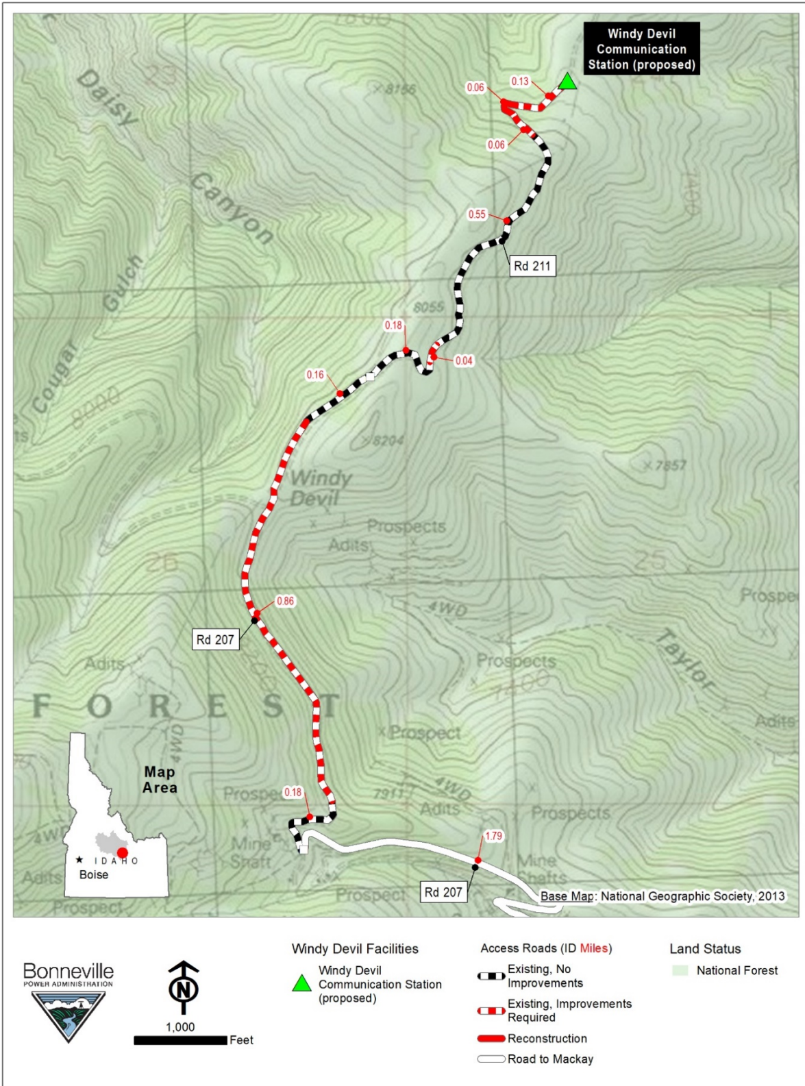
Figure 3. Windy Devil Communication Station Access Road Improvements
