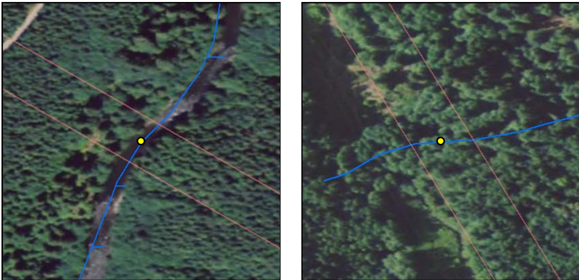
Figure 6. Example of high stream shade hazard at a fish-bearing stream crossing (left, crossing K-8) and low stream shade hazard (right, crossing 9-25). Scale 1:4,800.
