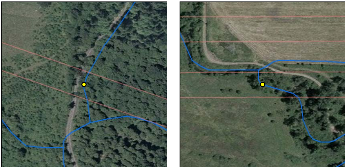
Figure 7. Examples of adjacent non-forest land use limiting to LWD recruitment potential and not to stream shade at a fish-bearing stream crossing (left, crossing M-2) and limiting to LWD recruitment potential and stream shade (right, crossing 36B-1). Scale 1:4,800.
