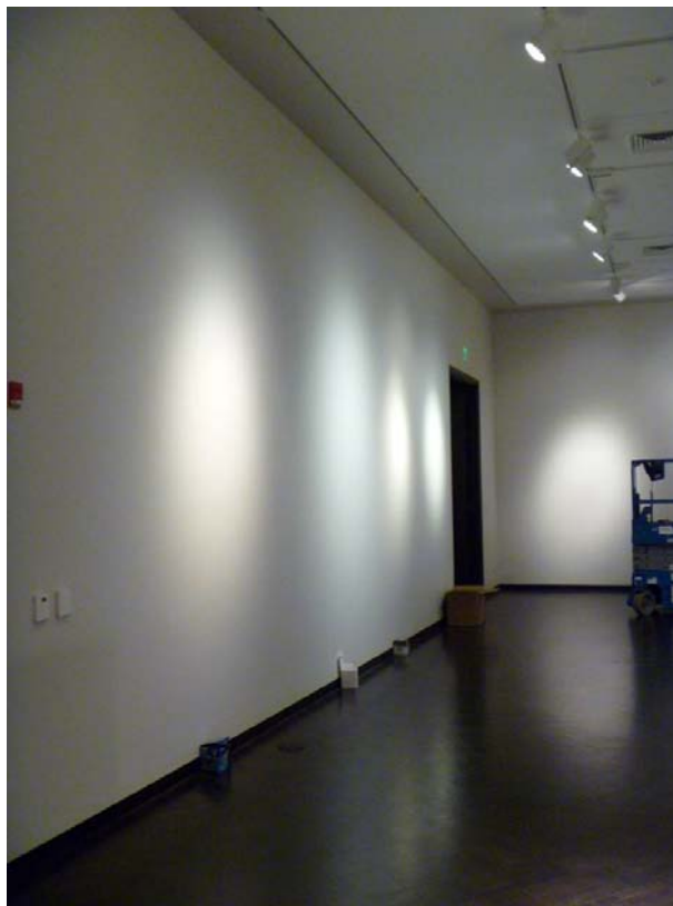
Figure 2. Mockup of four LED lamp types (left wall) in the Barker Gallery. The Cree PAR38 (“LRP38”) lamp is on the far left, nearest the viewer. The incumbent halogen lamp is projected on the far wall. There were no screens, louvers, or lenses in place to modify the projected beams in the track heads for this test. Notice the difference in color and beam edge among the different lamps.
