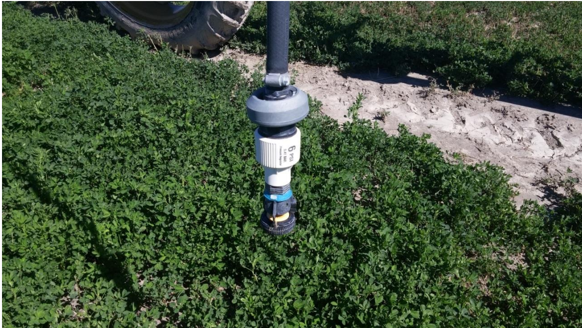
Figure 8. Weight, pressure regulator and spray head assembly for a LESA drop.
