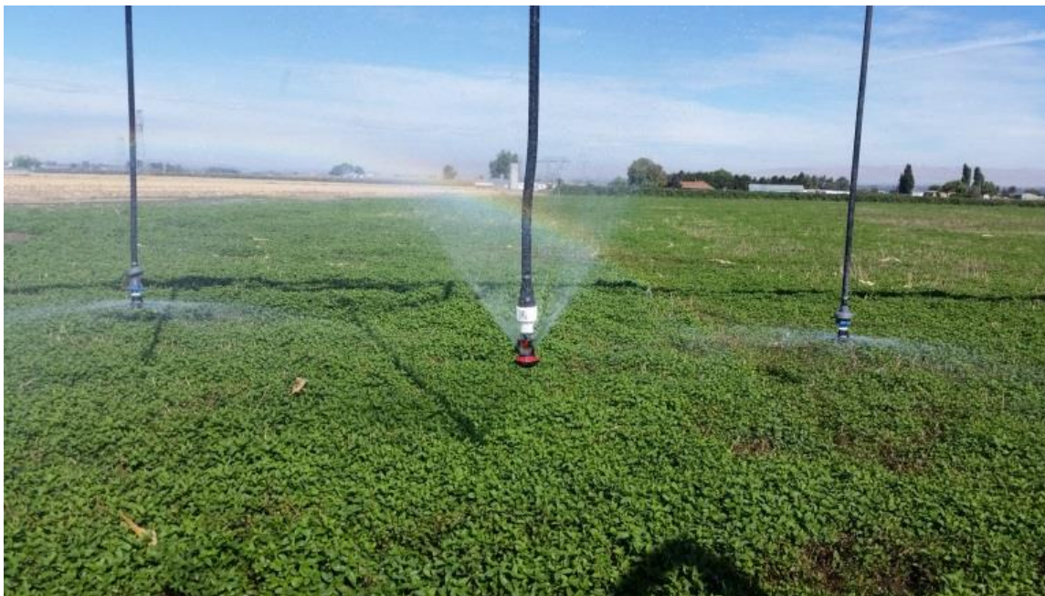
Figure 28. Chemigation plates can be used to spray water upwards to improve canopy wetting for chemigation.
