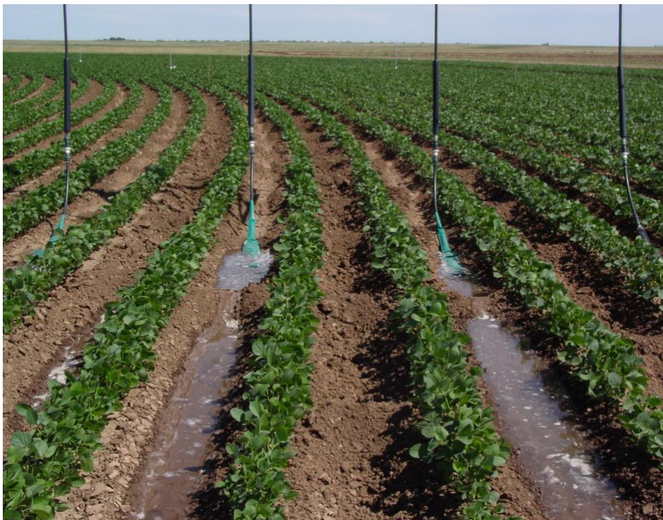
Figure 4. LEPA on a row crop using drag socks to minimize erosion to the furrow dikes that limit water movement in the furrows.
