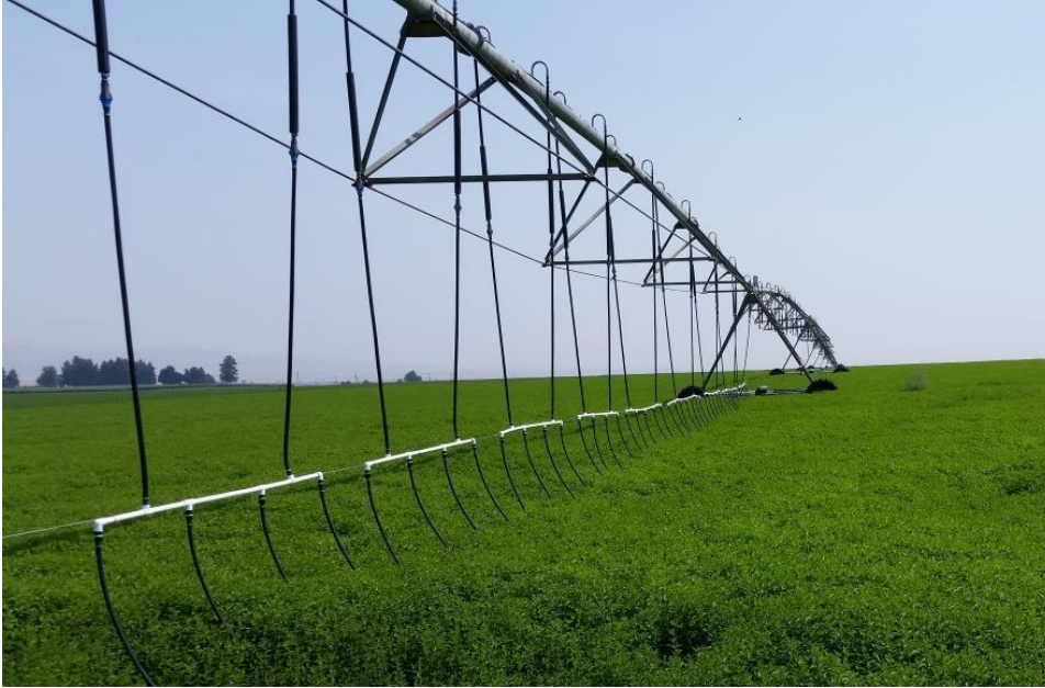
Figure 5. LEPA on mint. This setup allows conversion back to MESA for better crop germination if desired.
