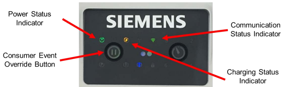
Figure 2-8 Visual Indicators and Controls on EVSE
