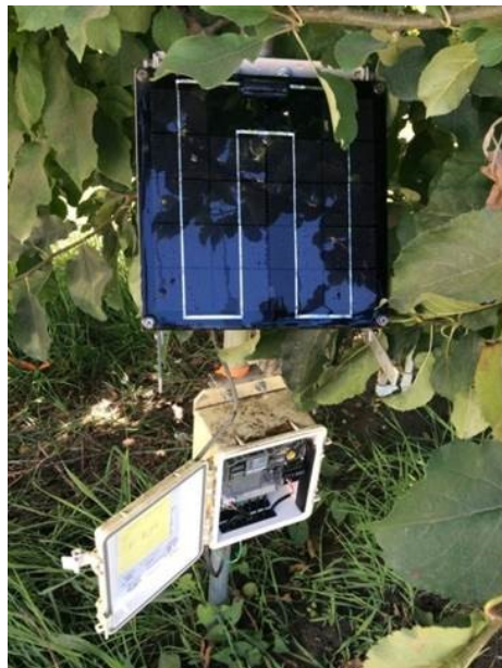
Figure 4: Example of a Partially Shaded Solar Panel—Could Impact Battery Charge
