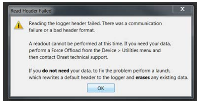
Figure 10: Error Message When Exporting Data from the Logger Affected by UV Light Exposure
