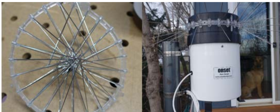
Figure 6: Bird-B-Gone Strip Before Assembly (left) and After Assembly (right)
