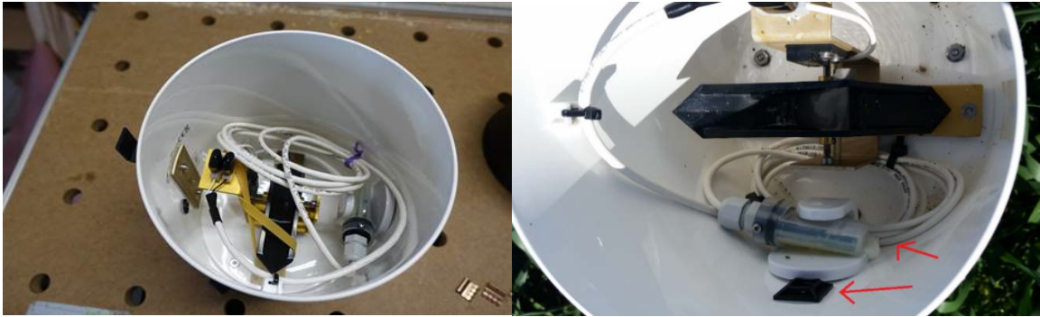
Figure 1: Example of Messy Cords (Left) and Clean Cords (Right) in a Tipping Rain Gauge
