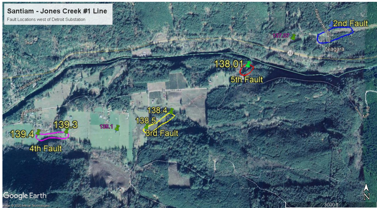
Figure 5 Locations of faults on the Jones Canyon-Santiam 230 kV line
