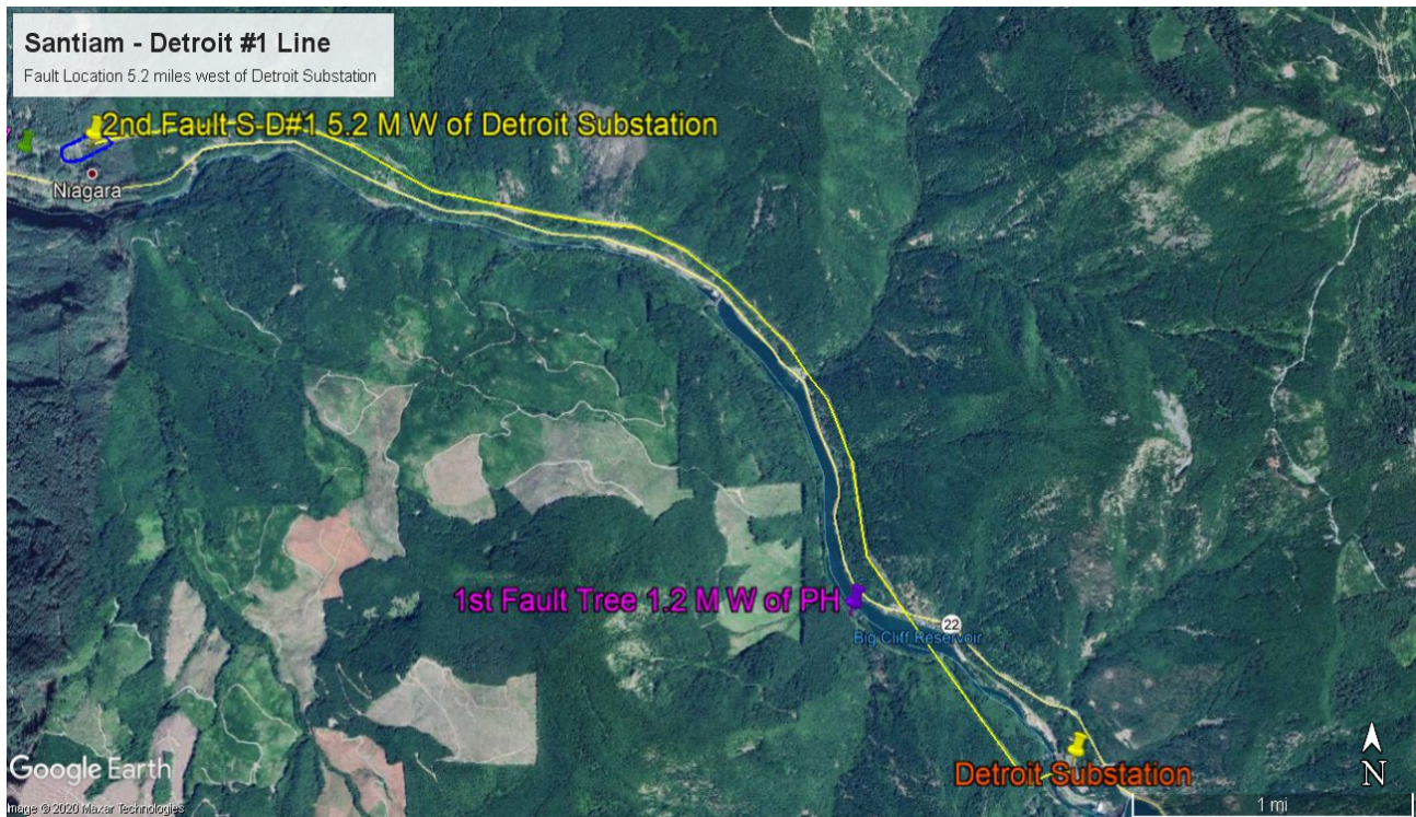
Figure 4 2 nd Fault location to the west and north of Niagara, no trees were found in the lines
