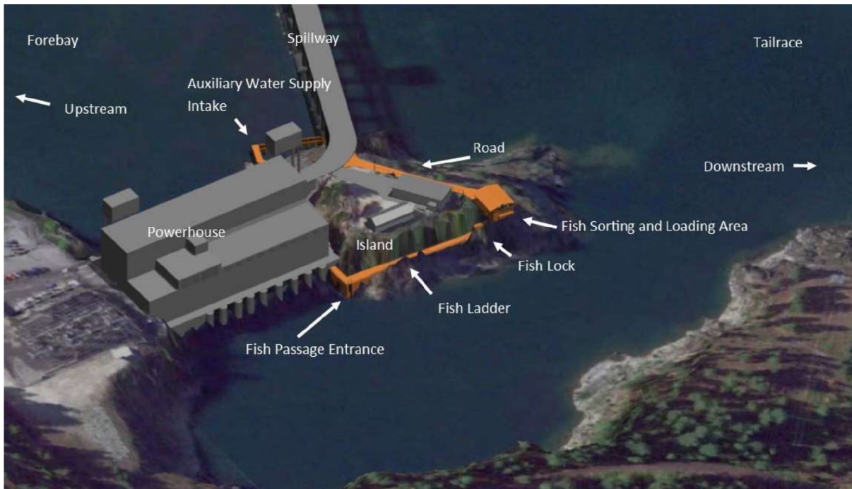
Figure 5-4. AFD Proposed Fish Passage Facility Layout (view from downstream side)
