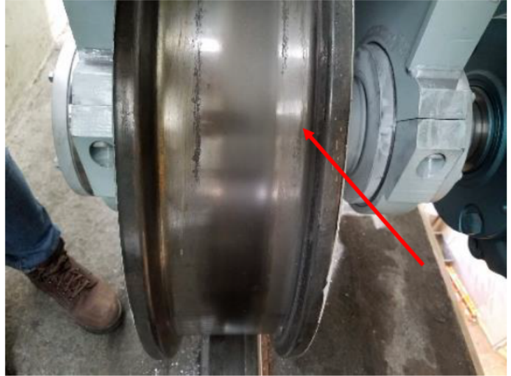
Photo 6: Wheel 2 Flange Visual Inspection (No Signs of Wear)
