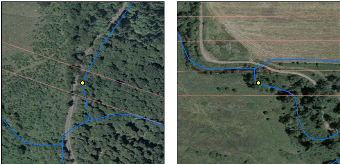
Figure 7. Examples of adjacent non-forest land use limiting to LWD recruitment potential and not to stream shade at a fish-bearing stream crossing (left, crossing M-2) and limiting to LWD recruitment potential and stream shade (right, crossing 36B-1). Scale 1:4,800.
