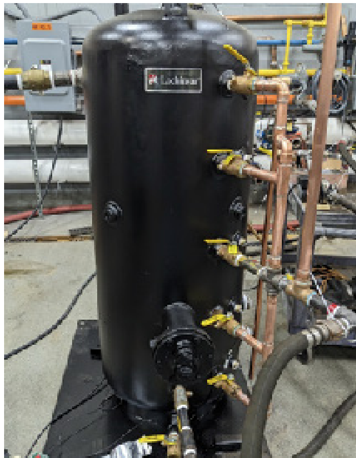
Figure 2-3. Storage tank configured with multiple inlet ports. During defrost testing, first the bottom port was used for defrost return, then the top port was used.
