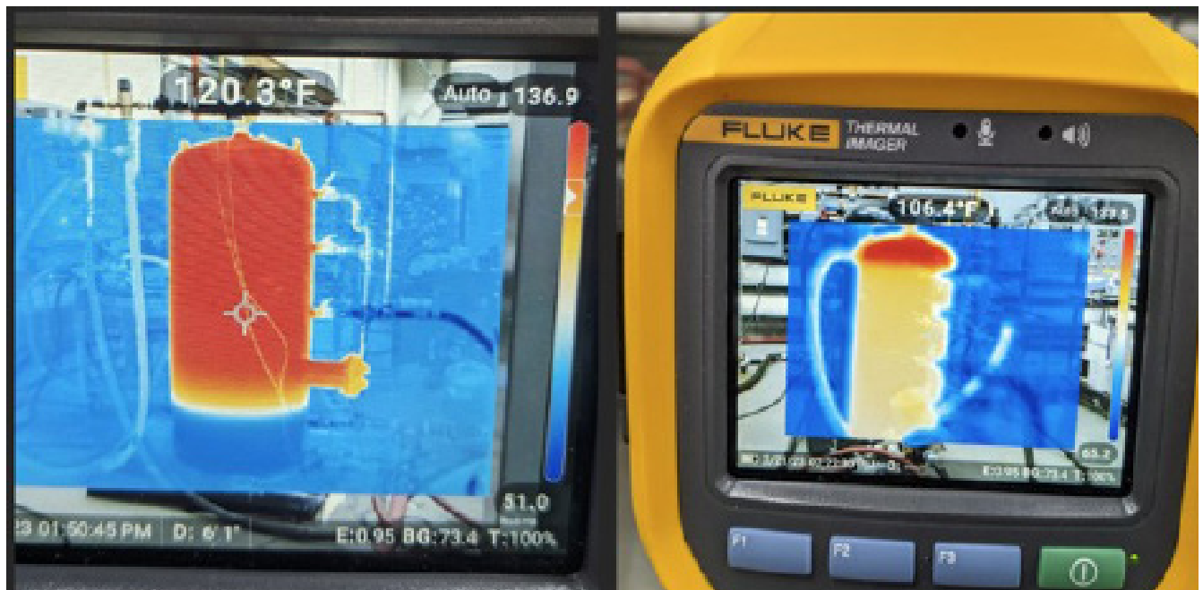
Figure 2-4. The left figure shows the storage tank at the end of the first defrost test, where the defrost water was piped back into the bottom of the tank. The storage tank is extremely well stratified for delivering hot water at 120°F. The right figure shows the storage tank at the end of the second defrost test. Almost no hot water is available above 120°F.
