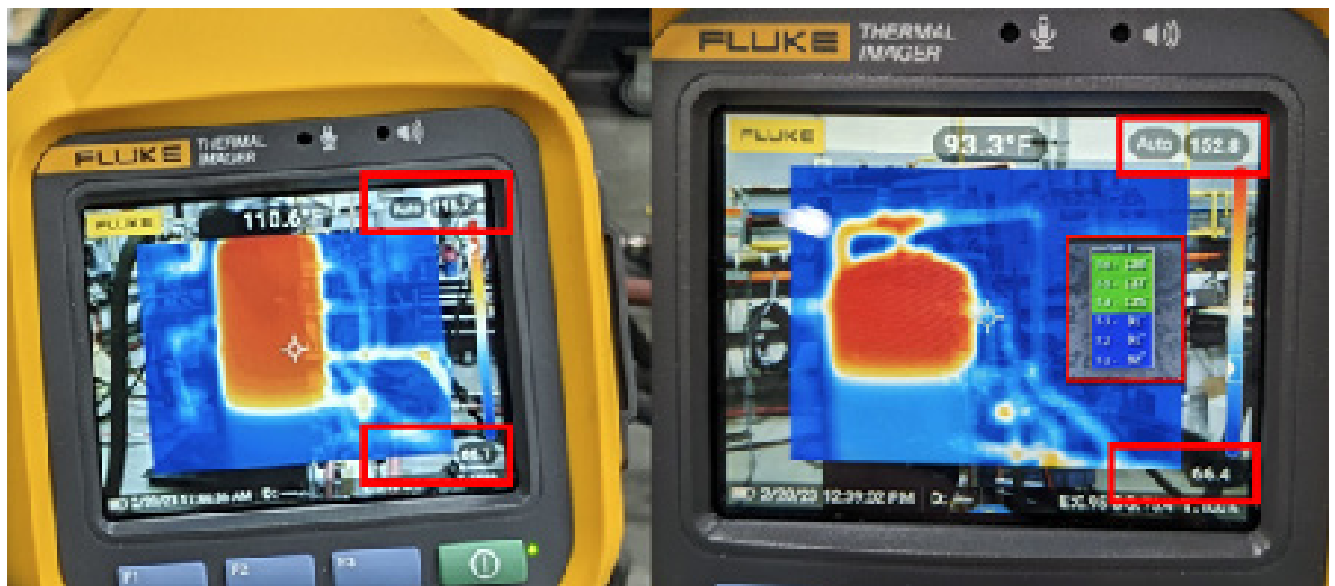
Figure 2-1. Formation of tank stratification. Note the difference in scale on the two images.
