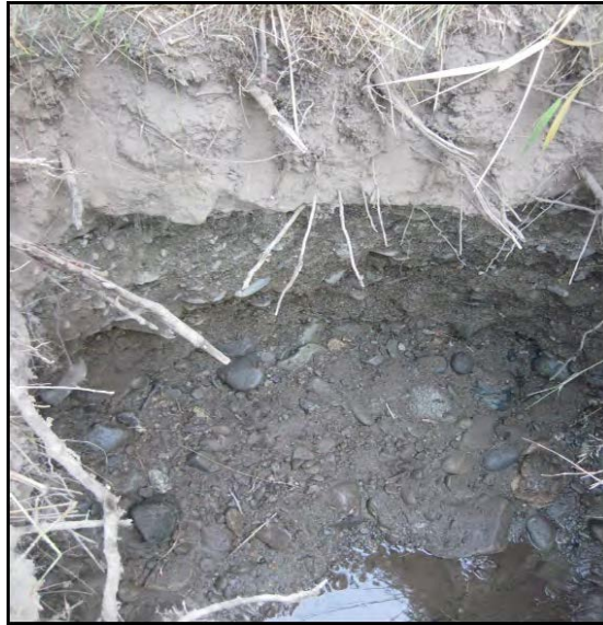
2017014: Newbry Meadows, Test pits dug showed a substrate profile consisting of sandy loam, sandy gravel, and clay.
