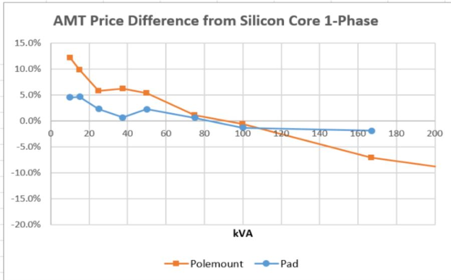
Figure 7. Incremental Costs for Single-Phase Pole and Pad-Mount ACT
