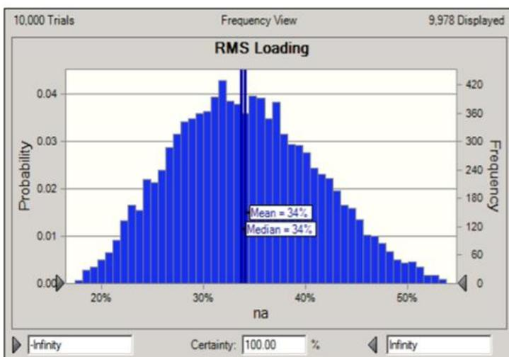
Figure 17. Average Loading on Utility-Owned Liquid-Immersed Distribution Transformers
