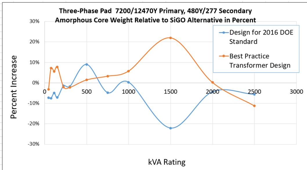
Figure 14. Weight of Three-Phase Pad-Mount ACT Compared to Conventional Silicon Steel Core Transformers
