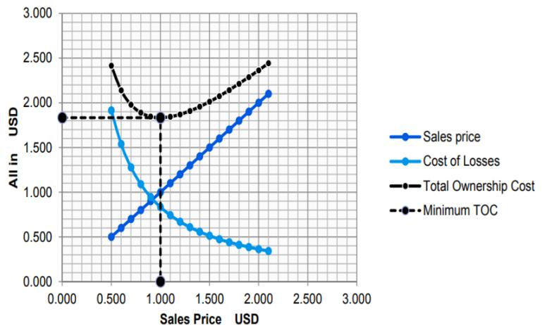
**Figure 5. Use of TCO Methodology to Select the Most Cost-Effective Transformer**
