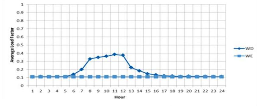
Figure 3. Typical Load Profile for a Commercial Sector Transformer on Weekdays (WD) and Weekends (WE)
