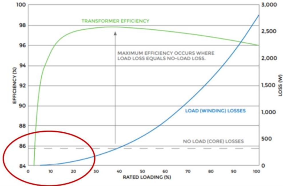
Figure 2. Impact of Load on Losses and Efficiency
