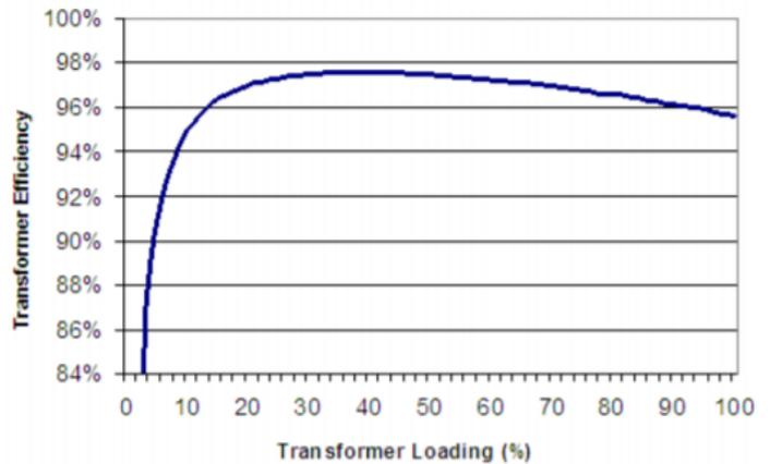
Figure 16. Transformer Efficiency Relative to Load
