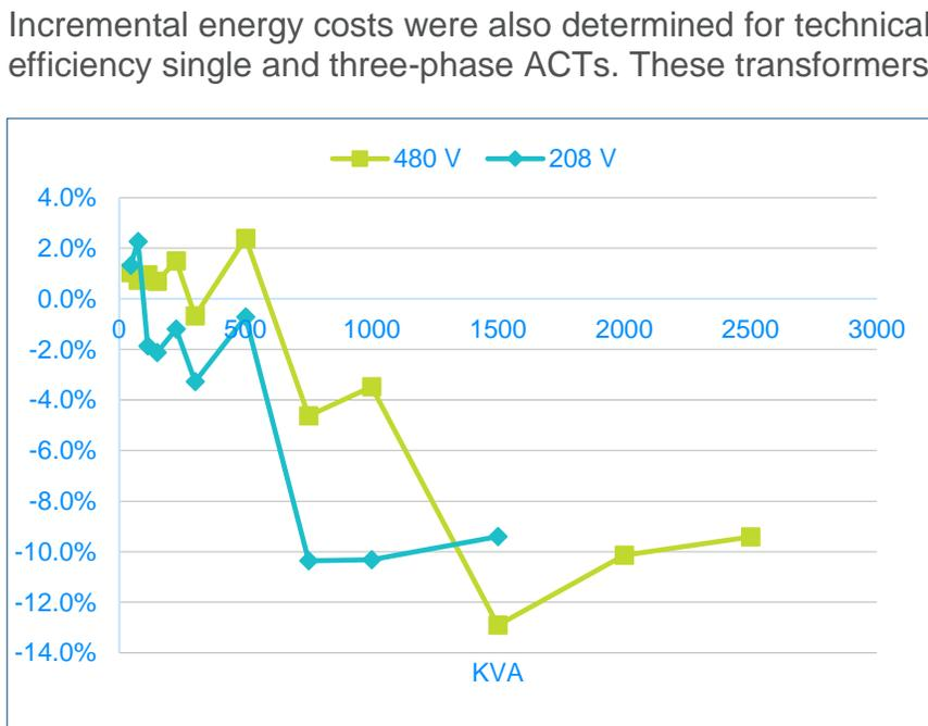
Figure 8. Three-Phase Pad-ACT Costs versus Baseline Transformers
