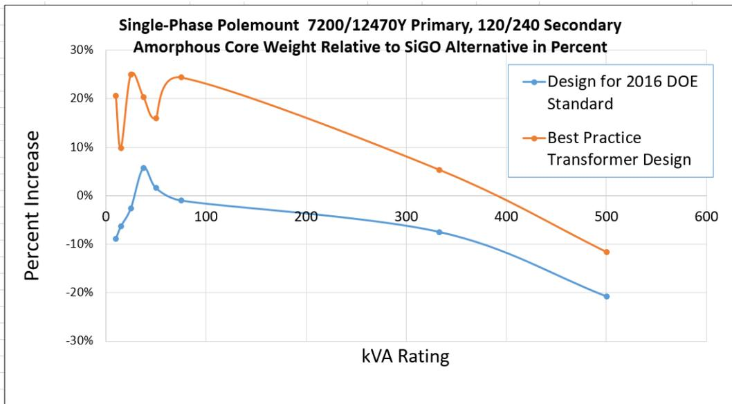
Figure 13. Weight of Single-Phase Pole-Mounted ACT Compared to Conventional Silicon Steel Core Transformers
