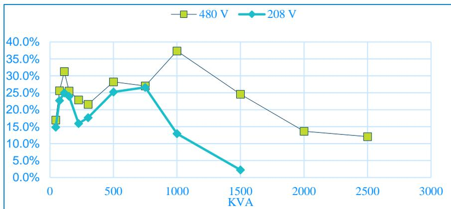
**Figure 10. Incremental Costs Enhanced Efficiency ACT Three-Phase Pad-Mount versus Baseline Transformers**
