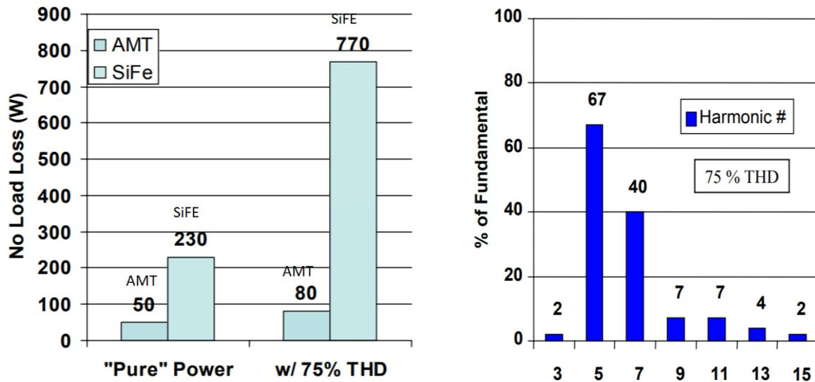
Figure 18. Laboratory Test Data Showing Impacts of Harmonic Distortion on No-Load Losses
