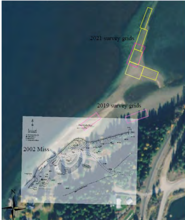
Figure H-2: Comprehensive map of magnetometry (yellow) and GPR (pink) survey efforts at 10BR100 (adapted from Maroney 2020).
