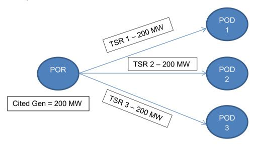
POR – Point of Receipt Cited Gen – Generation Facility Capability Cited in Data Exhibits POD – Point of Delivery TSR – Transmission Service Request
