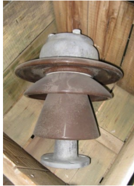
34.5kV Single Unit Cap & Pin
