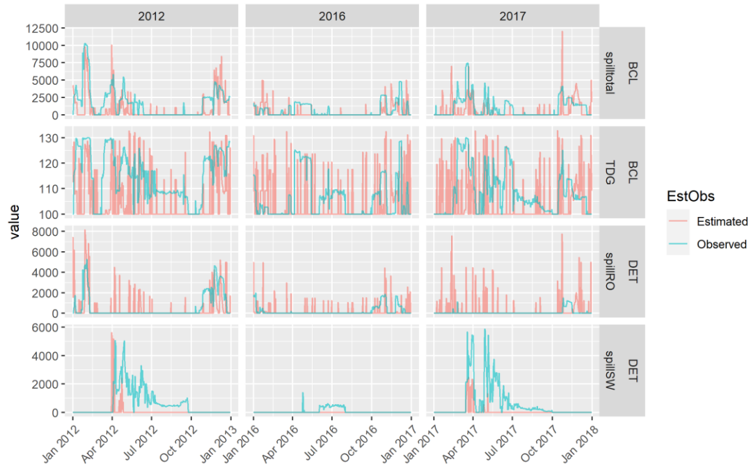
Figure 2-29. Simulated operations and TDG at Detroit (DET) and Big Cliff (BCL) During three relatively large spring-time flow events comparing NAA (Estimated) to observed historical data (Observed). Abbreviations: spillRO; Regulating Outlet spill flow, spillSW; Spillway outlet flow, spilltotal; Total outflow.
