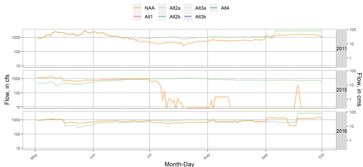
Figure 1-108. WV EIS HEC-ResSim Green Peter Dam Total Outflow in 2011, 2015, and 2016 Under Alternative 2a and NAA.
