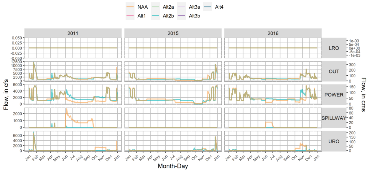
Figure 1-151. WV EIS HEC-ResSim Gate-Specific Outflows in 2011, 2015, and 2016 Under Alternative 2b and NAA.
