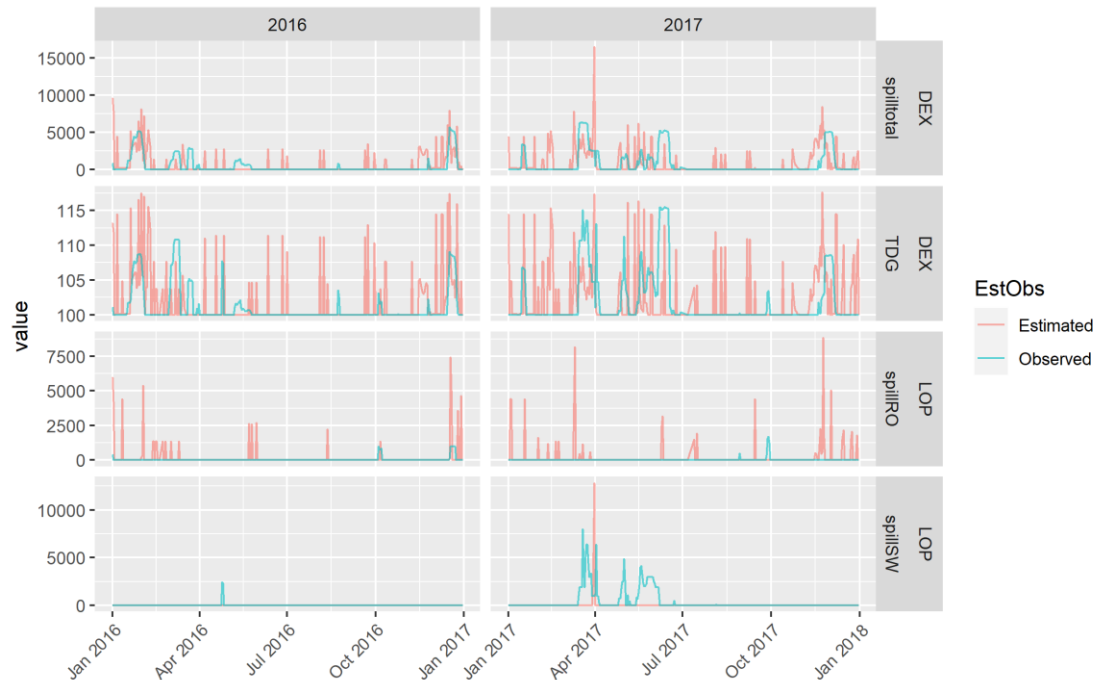
Figure 2-32. Simulated operations and TDG at Lookout Point (LOP) and Dexter (DEX) During two relatively large spring-time flow events comparing NAA (Estimated) to observed historical data (Observed). Abbreviations: spillRO; Regulating Outlet spill flow, spillSW; Spillway outlet flow, spilltotal; Total outflow.
