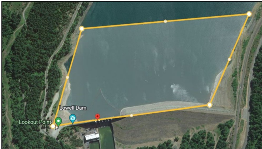
Figure 5-6. Lookout Point Dam Tailrace, Forebay, and Near Forebay Zone (gray) Showing Approximate Area to be Used for Measuring Fish Passage Metrics.
