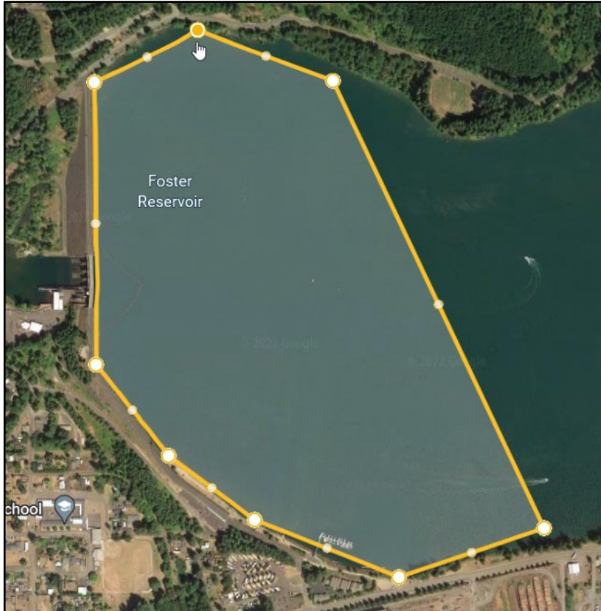
Figure 5-4. Foster Dam Tailrace, Forebay, and Near Forebay Zone (gray) Showing Approximate Area to be Used for Measuring Fish Passage Metrics.
