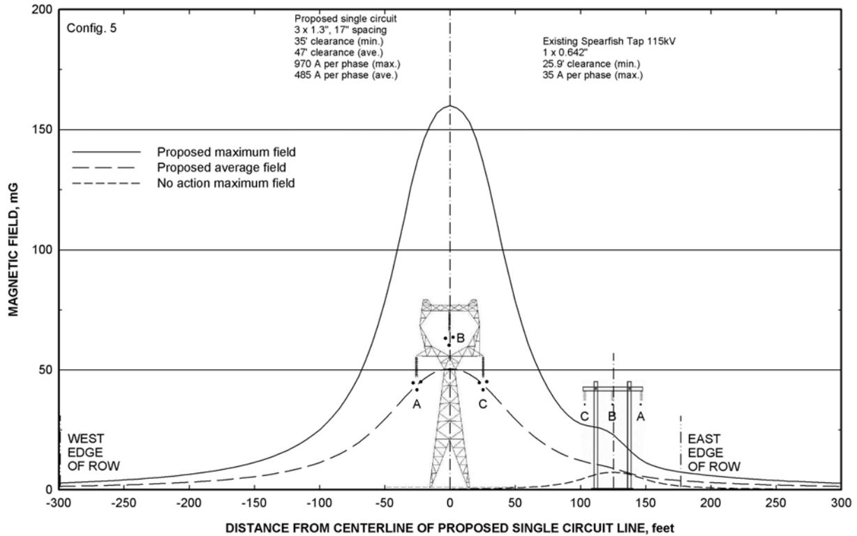
**Figure 30: Magnetic-field profiles for single-circuit Configuration 6 of the proposed Big Eddy – Knight 500-kV line.** Fields computed for maximum current with minimum clearance and for average current with average clearance are shown. Configurations are described in Tables 1 and 2.
