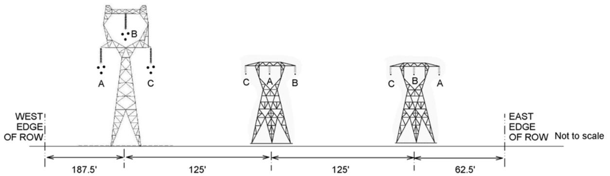
**Figure 5: Single-circuit Configuration 4 for the proposed Big Eddy – Knight 500-kV line.** Configurations are described in Tables 1 and 2.
