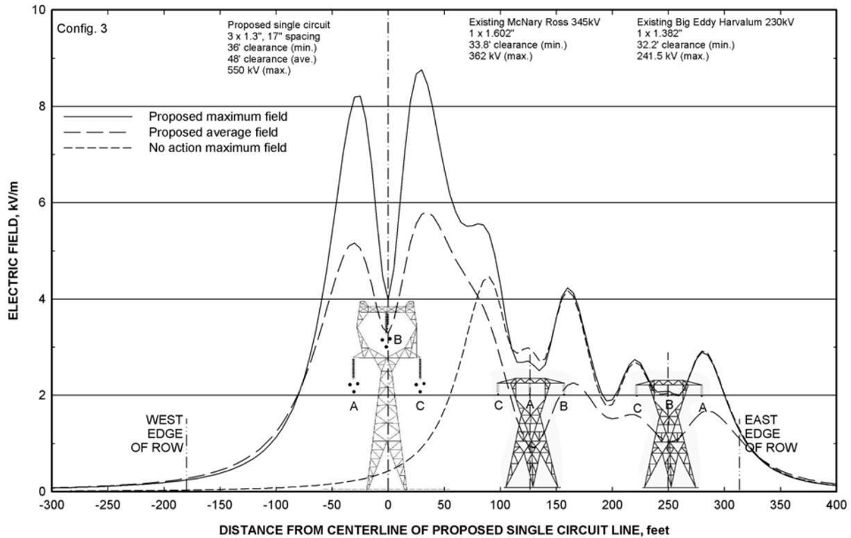
**Figure 16: Electric-field profiles for single-circuit Configuration 4 of the proposed Big Eddy – Knight 500-kV line:** Fields for maximum voltage with minimum and average clearances are shown. Configurations are described in Tables 1 and 2.
