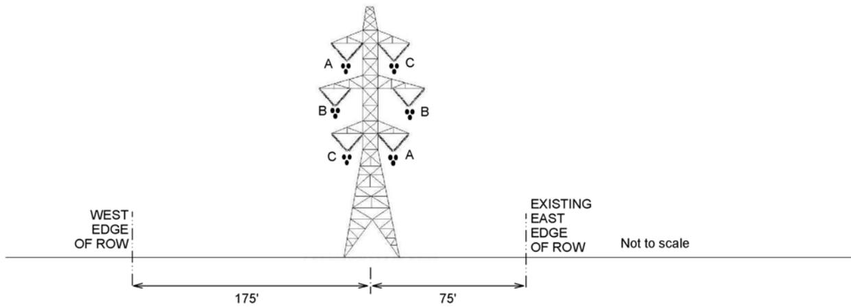
**Figure 10: Double-circuit Configuration 9 for the proposed Big Eddy – Knight 500-kV line.** Configurations are described in Tables 1 and 2.
