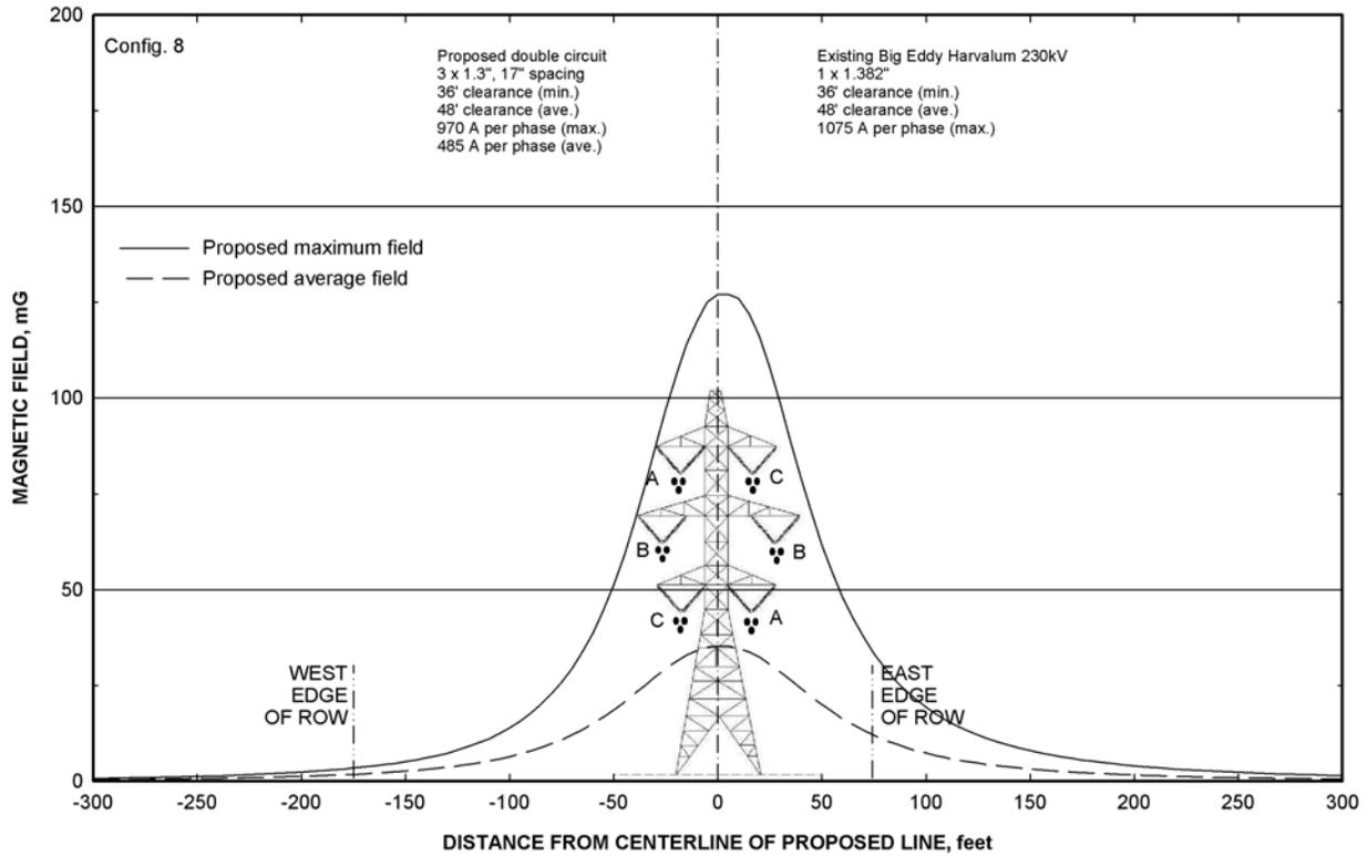
**Figure 33: Magnetic-field profiles for double-circuit Configuration 9 of the proposed Big Eddy – Knight 500-kV line.** Fields computed for maximum current with minimum clearance and for average current with average clearance are shown. Configurations are described in Tables 1 and 2.
