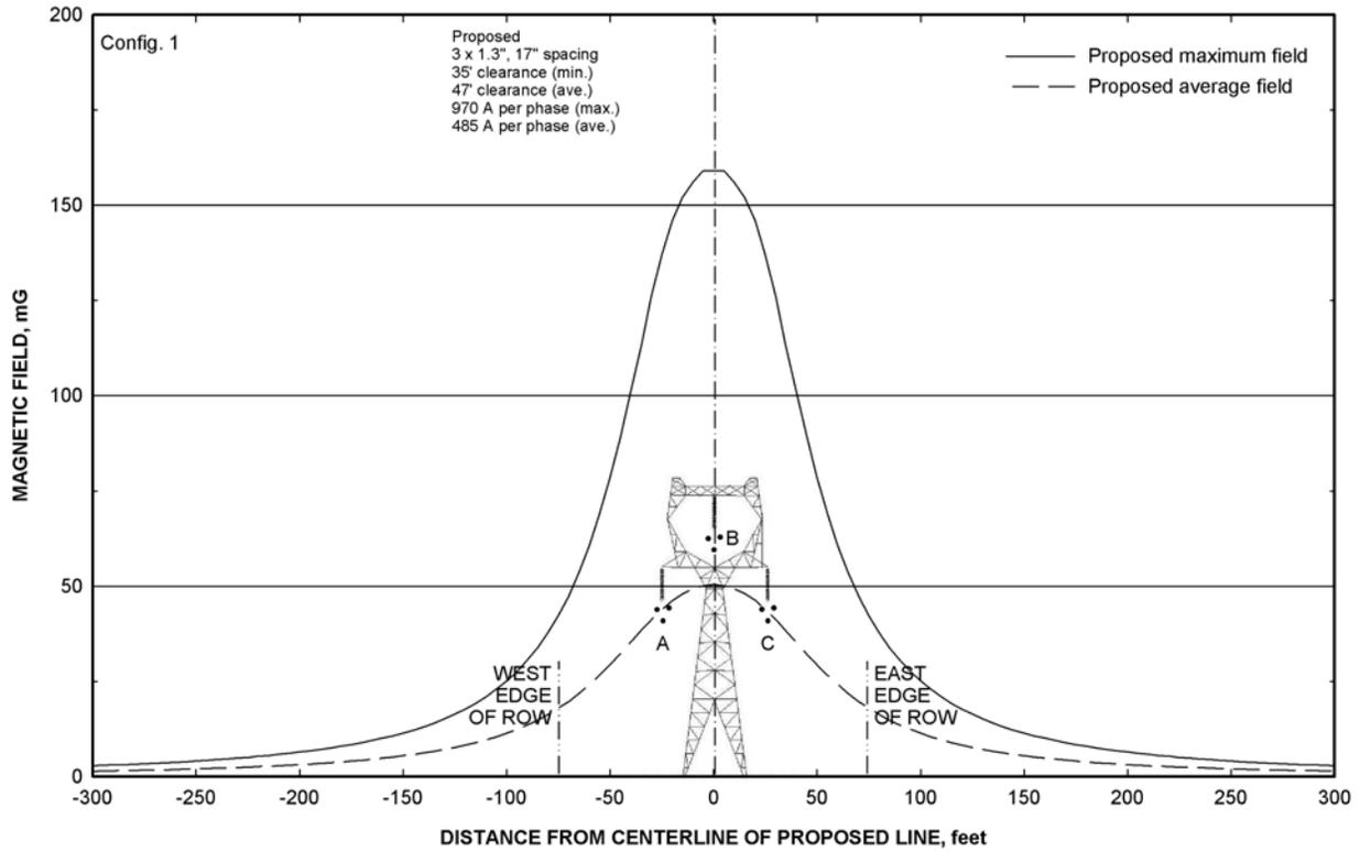
**Figure 26: Magnetic-field profiles for single-circuit Configuration 2 of the proposed Big Eddy – Knight 500-kV line.** Fields computed for maximum current with minimum clearance and for average current with average clearance are shown. Configurations are described in Tables 1 and 2.
