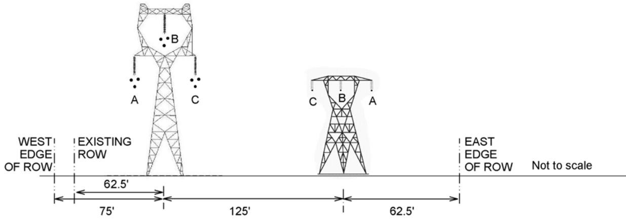
**Figure 4: Single-circuit Configuration 3 for the proposed Big Eddy – Knight 500-kV line.** Configurations are described in Tables 1 and 2.
