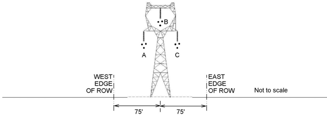
**Figure 3: Single-circuit Configuration 2 for the proposed Big Eddy – Knight 500-kV line.** Configurations are described in Tables 1 and 2.
