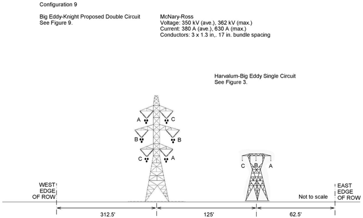
**Figure 11: Double-circuit Configurations 10 and 11 for the proposed Big Eddy – Knight 500-kV line.** The west circuit will be the proposed Big Eddy – Knight line and the east circuit will be the existing Chenoweth – Goldendale line (Configuration 10) or the existing Spearfish Tap line (Configuration 11). Configurations are described in Tables 1 and 2.
