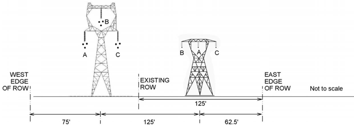
**Figure 8: Double-circuit Configurations 7 and 7A for the proposed Big Eddy – Knight 500-kV line.** The current is split between the two circuits in Configuration 7. The current is only on the west circuit in Configuration 7A and the east circuit conductors carry zero current and are not grounded. Configurations are described in Tables 1 and 2.
