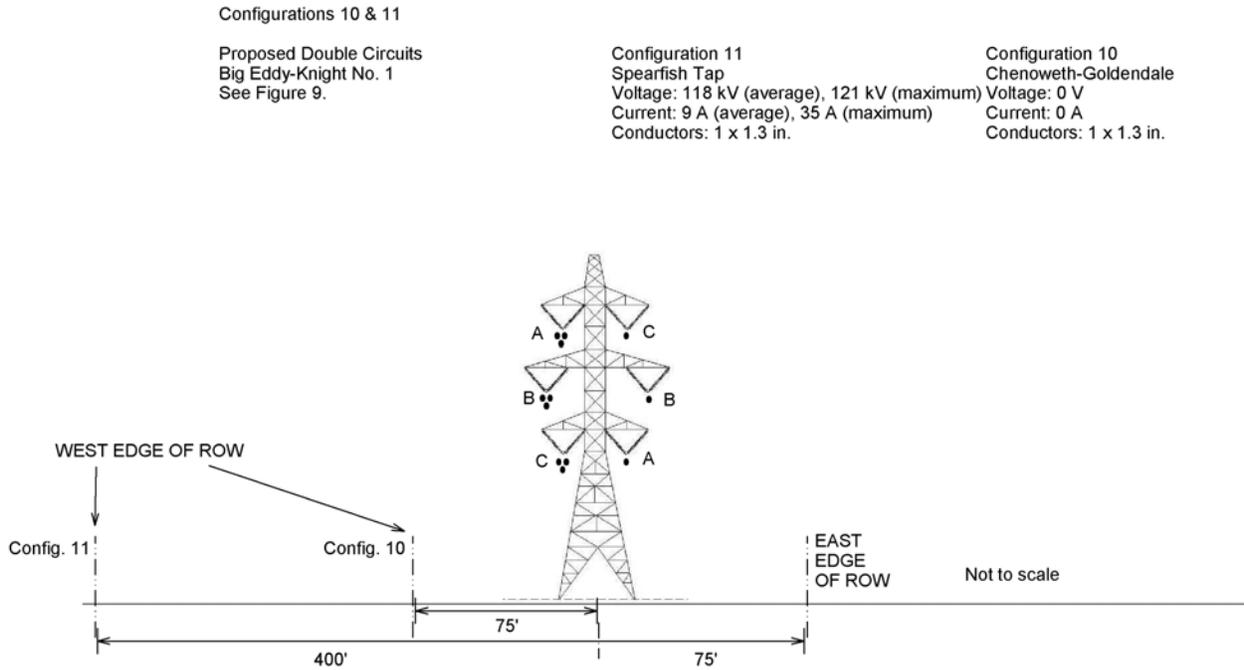
**Figure 12: Double-circuit Configuration 12 for the proposed Big Eddy – Knight 500-kV line.** Configurations are described in Tables 1 and 2.
