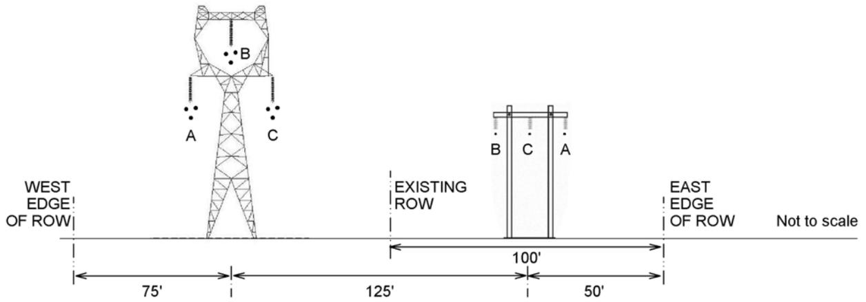
**Figure 6: Single-circuit Configuration 5 for the proposed Big Eddy – Knight 500-kV line.** Configurations are described in Tables 1 and 2.
