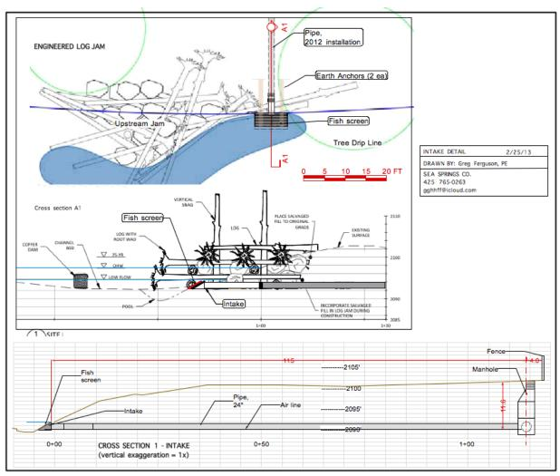
Figure 2-2. Surface Water Intake Design
