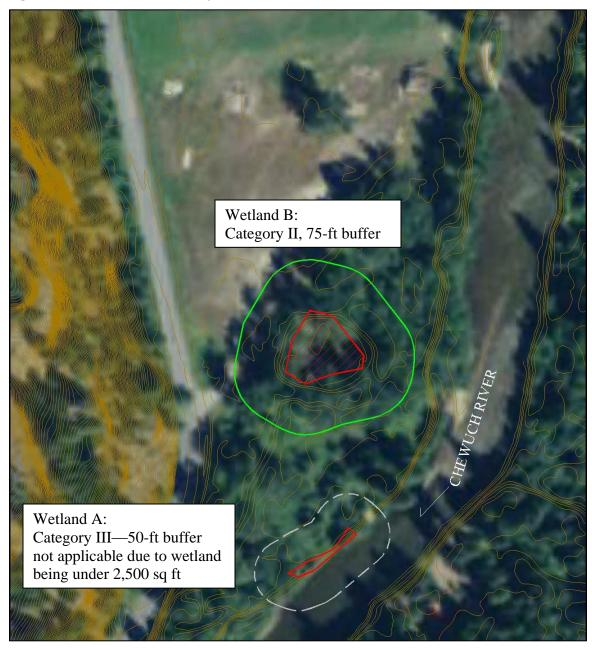
Figure 2. Wetland survey overlaid on hillshade survey data.
