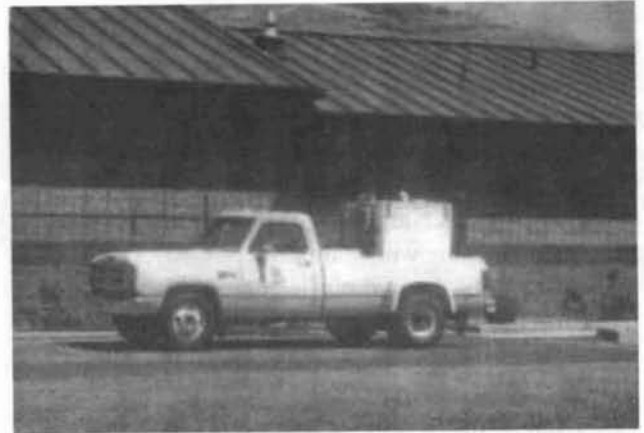
Figure 1-9. One of three 150 gal fish transport trucks used in the juvenile fish transportation program
