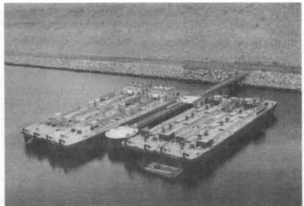
Figure 1-7. Fish barges (two 86,000 gal, two 100,000 gal, and two 150,000 gal capacity) used in the juvenile fish transportation program.
