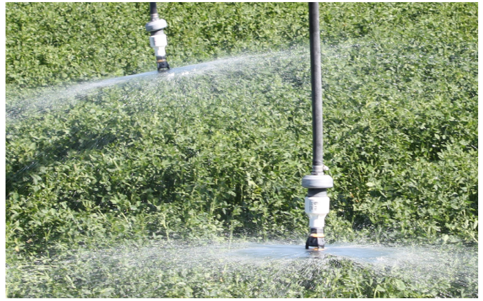
This LESA irrigation conversion installed in Eastern Washington uses less electricity than traditional sprinklers and reduces water waste from evaporation.
