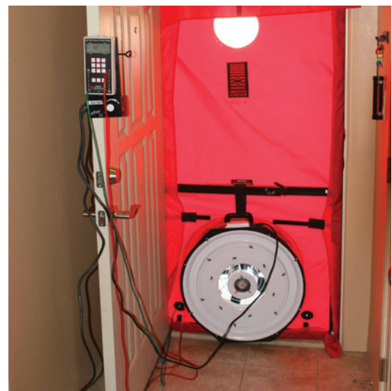
Blower door test: Air barriers are tested during a blower-door test, with the house at a pressure of -50 Pascals with reference to outdoors. This house has 2800 CFM 50 of air leakage.
