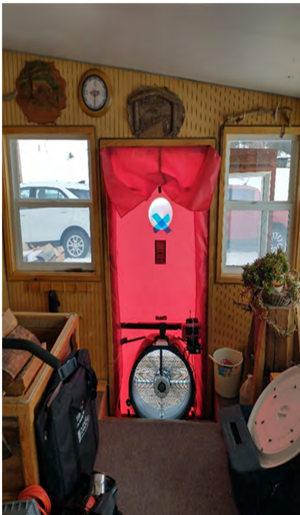
Figure 3. Blower Door test in Progress.
