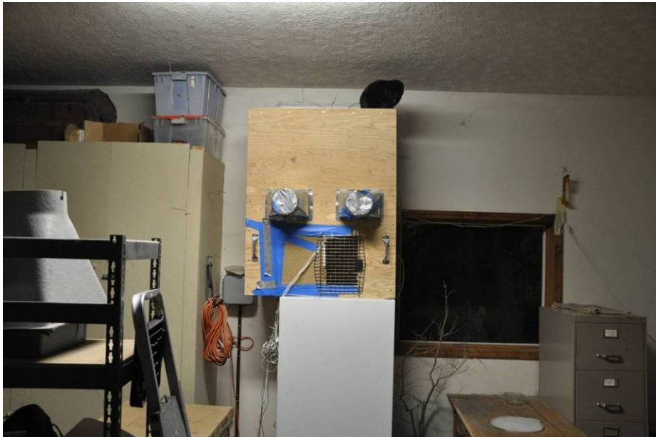
Figure 1. Head-on View of Indoor Unit Test Enclosure
