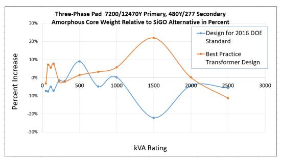
Figure 14. Weight of Three-Phase Pad-Mount ACT Compared to Conventional Silicon Steel Core Transformers
