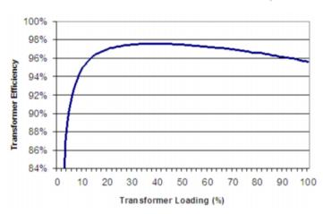
Figure 16. Transformer Efficiency Relative to Load
