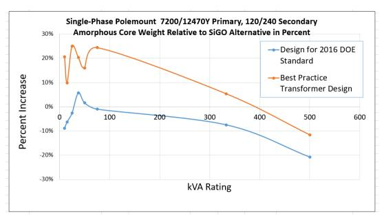
Figure 13. Weight of Single-Phase Pole-Mounted ACT Compared to Conventional Silicon Steel Core Transformers
