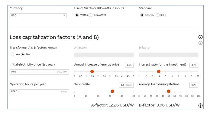
Figure 6. TCO Loss Multiplication Factor Calculator
