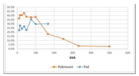
Figure 9. Single-Phase Pad and Pole-Mount Enhanced Efficiency ACT Incremental Costs versus Baseline GO Si-Steel Transformer
