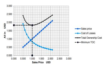
Figure 5. Use of TCO Methodology to Select the Most Cost-Effective Transformer
