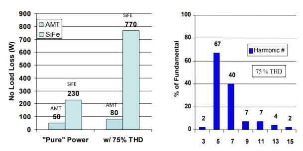
Figure 18. Laboratory Test Data Showing Impacts of Harmonic Distortion on No-Load Losses
