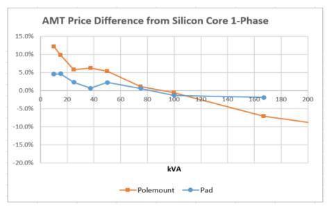
Figure 7. Incremental Costs for Single-Phase Pole and Pad-Mount ACT
