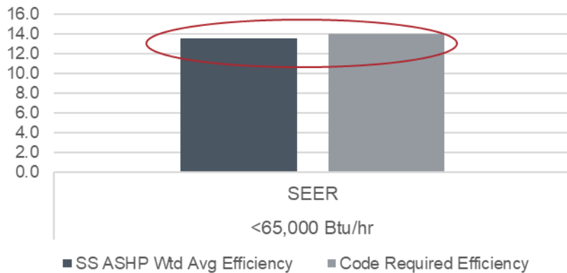
Split System ASHP Cooling Efficiency vs Code
