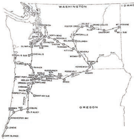
BPA's Microwave Radio Communication System in 1957.
