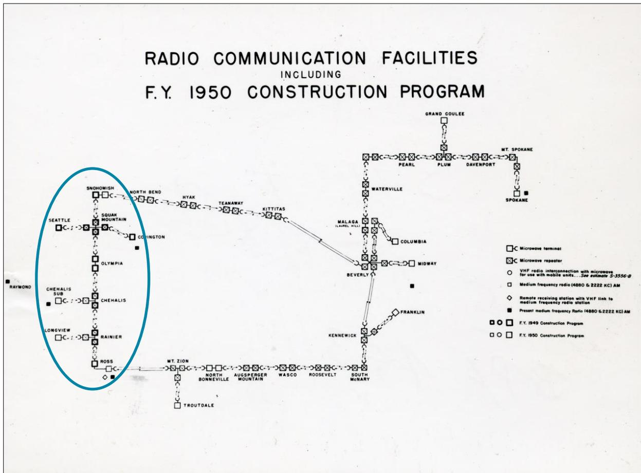
**Figure 33. Diagram showing BPA's Microwave Radio System Plan in 1950, highlighting the initial construction period.**
