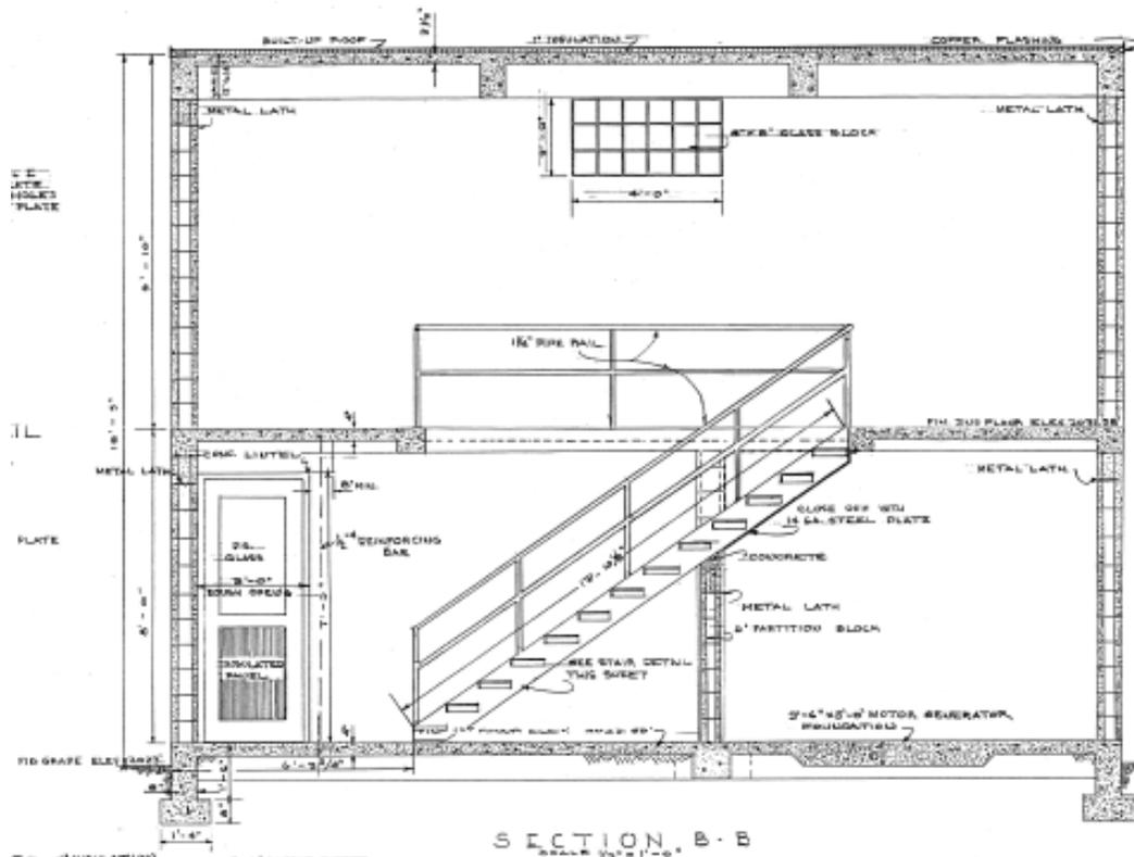
**Figure 40. Section drawing for Type 1602 Squak Mountain Radio Station Building, 1949 (BPA)**
