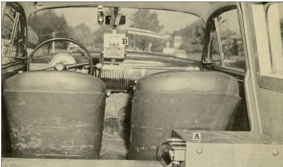
**Figure 11.** Survey car installation of VHF radio equipment for mobile field units, 1951 . A is the radio transmitter/receiver unit; B is the control head and field strength meter, with attached handset (BPA ECDU 1951).
