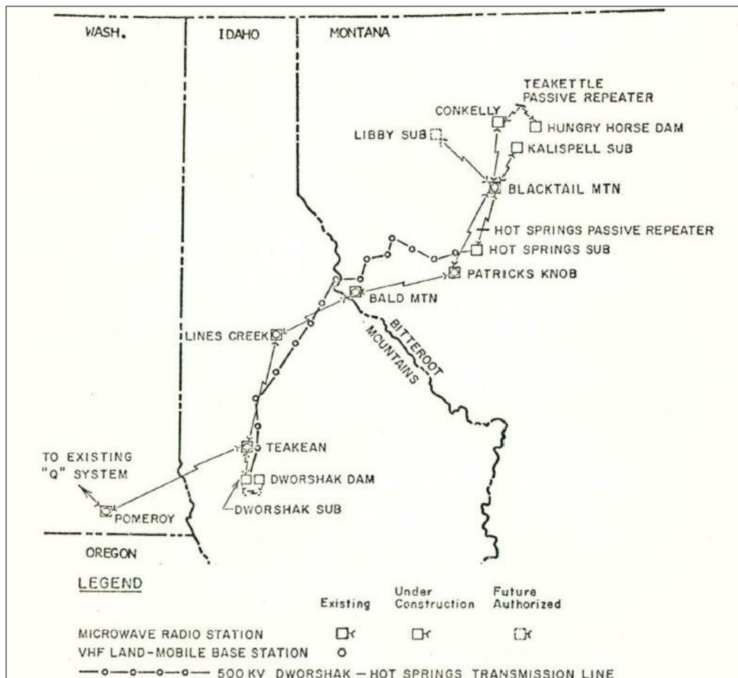
**Figure 37. BPA's "Q" Microwave System Extension to Idaho and Montana**
