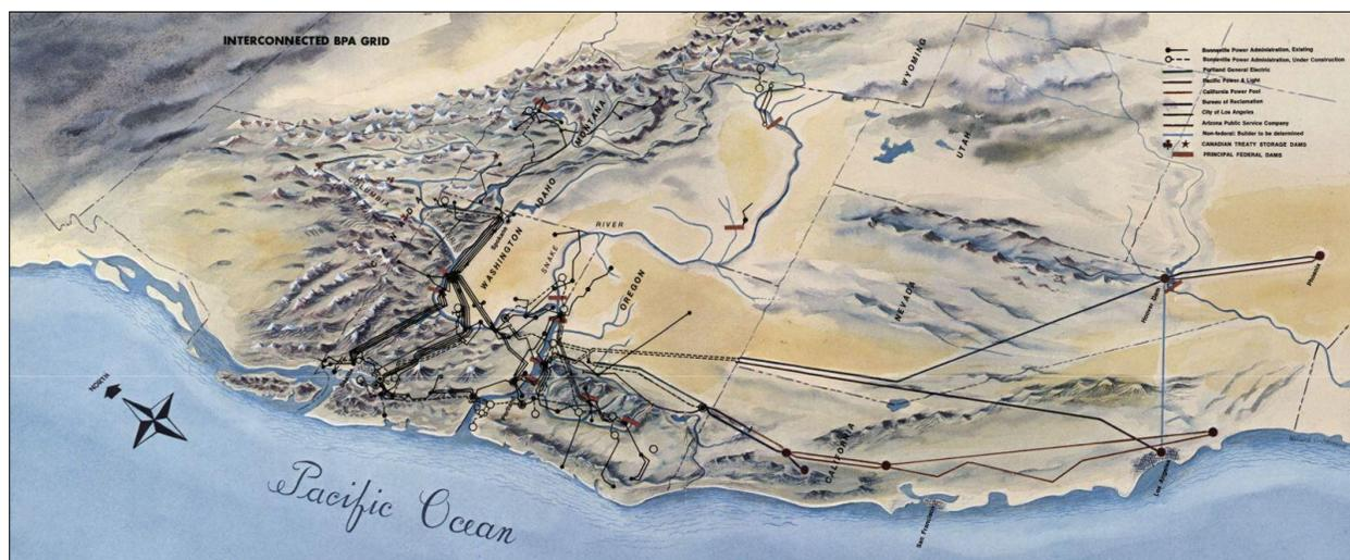
**Figure 26. Illustration of the BPA Grid, including the Intertie extending into California and Nevada (BPA 1966). The Intertie connected various types of transmission facilities with the Columbia River’s federal dams, including power, compensation, and converter stations. System functioning required a reliable communication system.**
