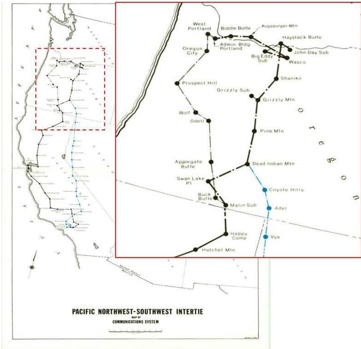
**Figure 36. Pacific Northwest - Southwest Intertie map with inset showing BPA's microwave radio sites**
