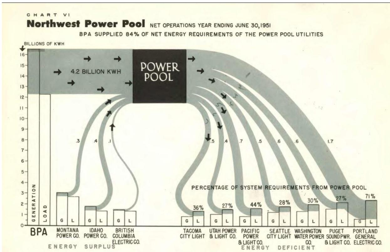
**Figure 6. Northwest Power Pool net operations for Fiscal Year 1950, illustrating the interconnected nature of operations between BPA and other power pool members (BPA 1951:28).**
