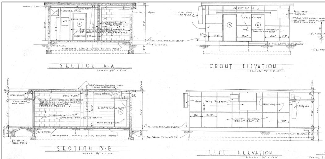
Figure 48. Elevation and drawings for Tacoma Microwave Radio Station Building, 1954 (BPA)
