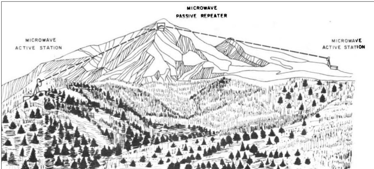
**Figure 1. This drawing illustrates principles of microwave technology related to line of sight, repeaters, and passive repeaters. Here, the “microwave passive repeater” overcomes the line of sight obstacle, an intervening mountain, to reflect transmissions between adjacent radio stations (BPA 1977:V-27).**
