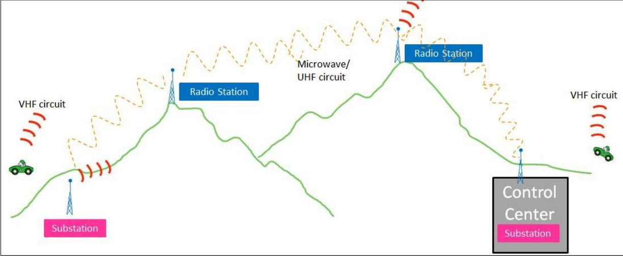
**Figure 2. Illustration of communication via microwave/UHF circuits and VHF circuits, showing transmission between two end locations. The sites use “line of sight propagation between antennas mounted to towers to receive and transmit those communications. The system also enables communication between a mobile unit and an end location and between two mobile units using mobile equipment and VHP whip antennas mounted on radio station antenna towers (BPA 1977:V-27).**
