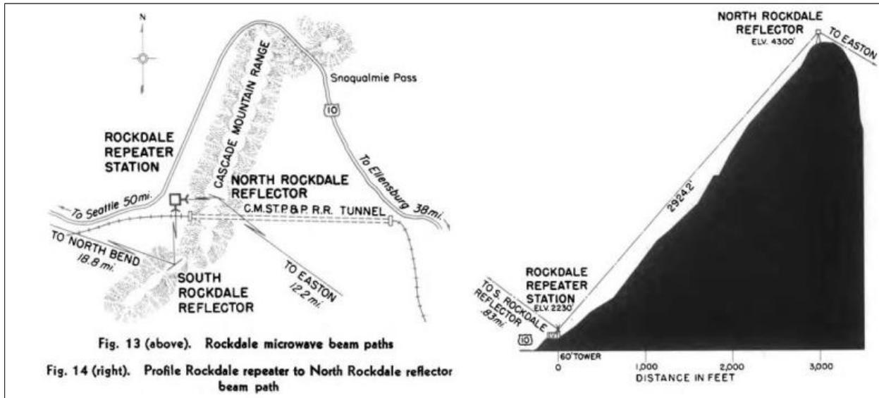
Figure 19. Rockdale Radio Station repeater scheme (Strong et al. 1957:659). The Rockdale radio station's transmissions are reflected by the North Rockdale reflector to Easton and by the South Rockdale repeater to North Bend.
