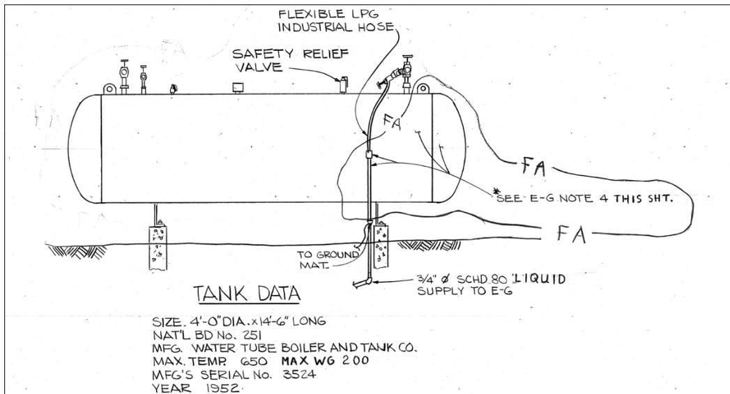
**Figure 73. Tank Drawing, Teanaway Microwave/Radio Station, redrawn in 1956 from 1953 original drawing (BPA)**
