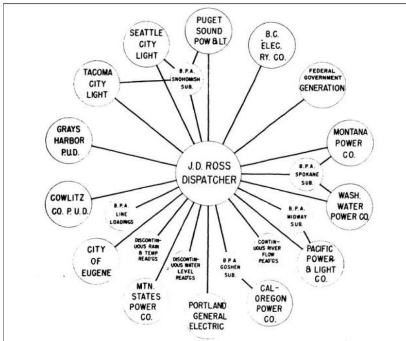
**Figure 7. BPA’s telemetry program schematic, centered at the J.D. Ross Complex, showing interconnections with BPA power substations and Northwest Power Pool members (Stevens and Stringfield 1951:32).**
