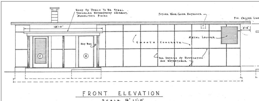
**Figure 45. Elevation Drawing for Type 1607 Kennewick Microwave Radio Station, 1952 (BPA)**
