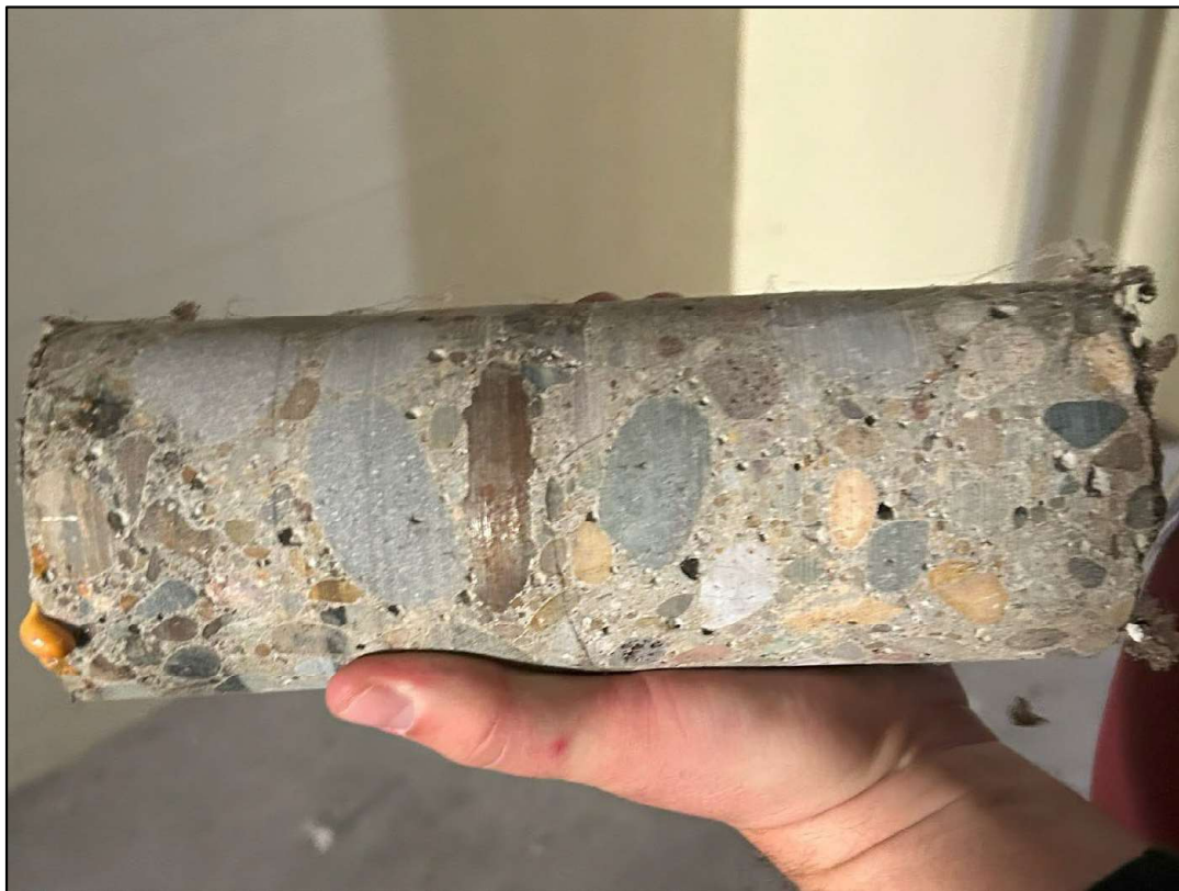
Photograph 36 of 46: OR_PolkCounty_SalemSubstation_0036 9in cored portion of reinforced Control House wall (2024)
