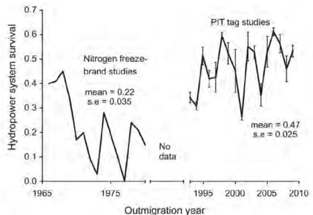
Fig. 4. Hydropower system Chinook salmon smolt (wild and hatchery combined) survival (from the uppermost dam to Bonneville Dam) estimated from nitrogen freeze-brand studies in the 1960s and 1970s prior to complete hydropower system development and from PIT tags studies (Snake River trap above Lower Granite Dam to the tailrace of Bonneville Dam) since 1993. Standard errors are shown for the PIT tag estimates.
