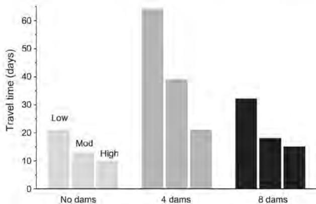
Fig. 5. Hydropower system Chinook salmon travel time (days) from Lower Granite (Rkm 695) to Bonneville Dam (Rkm 234) under low (Snake 995–1505, Columbia 4005–5028 m<sup>3</sup> s<sup>-1</sup>), moderate (Snake 2017–3010, Columbia 6022–9034 m<sup>3</sup> s<sup>-1</sup>), and high (Snake 4010–5028, Columbia 10,028–14,034 m<sup>3</sup> s<sup>-1</sup>) flow conditions with no dams, 4 dams, and 8 dams.
