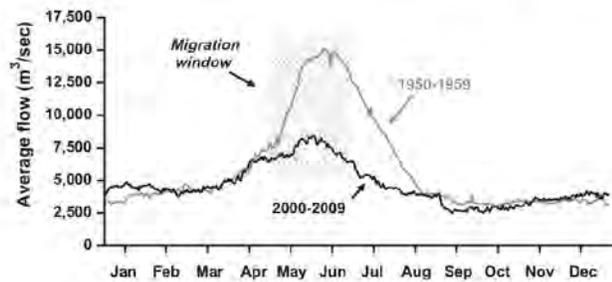
Fig. 2. Ten-year average flow ( $\text{m}^3 \text{s}^{-1}$ ) measured at Bonneville Dam before (1950–1959) and after full hydropower system development. The downstream migration period for stream-type Chinook salmon is also shown.
