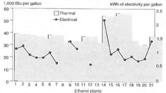
Ethanol plants use natural gas to produce steam to convert corn to ethanol. On average, the surveyed ethanol plants used 34,800 Btu of thermal energy per gallon of ethanol. Thermal energy used per gallon of ethanol varied among ethanol plants and ranged from 26,000 to 54,000 Btu per gallon in 2002 (fig. 7).
