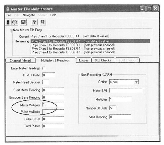
Figure 15 New Master File Entry—Multipliers & Readings
