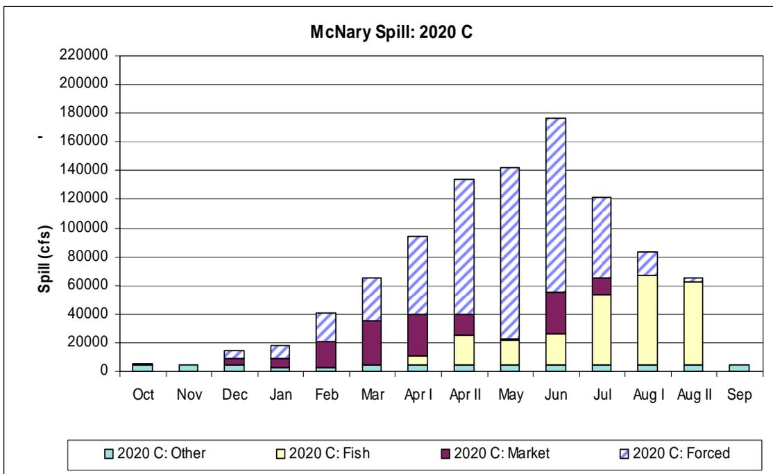
Figure 155. 2020 C Scenario: McNary Spill Breakdown.
