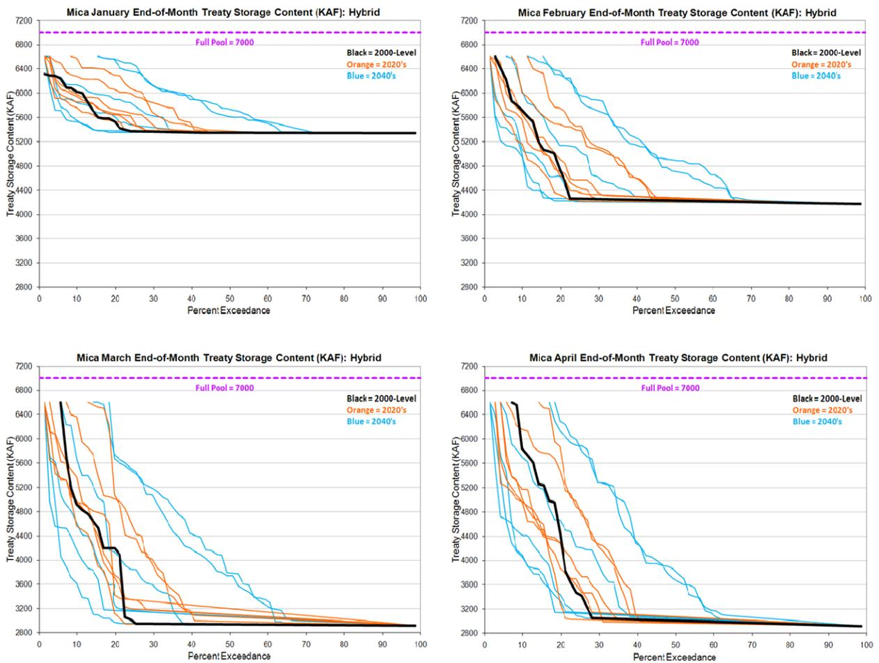
Figure 27. Mica Flood Control Storage Exceedance – Hybrid-Delta.
