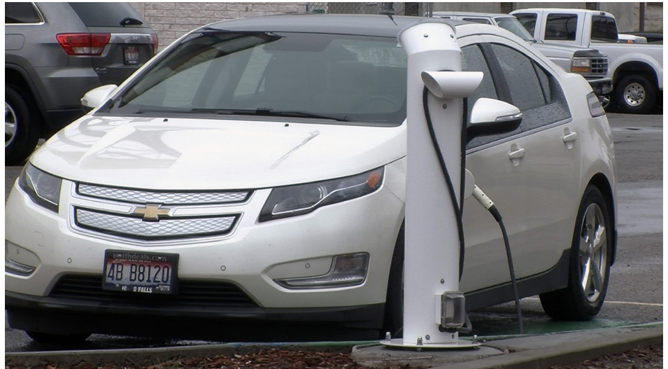
An electric vehicle charges using stored energy from a nearby photovoltaic panel.
