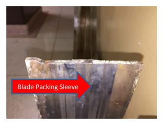
Photo 4 – Extreme Close-up of Blade Packing Sleeve after Removal from Unit Shows Fatigue on Left Side
