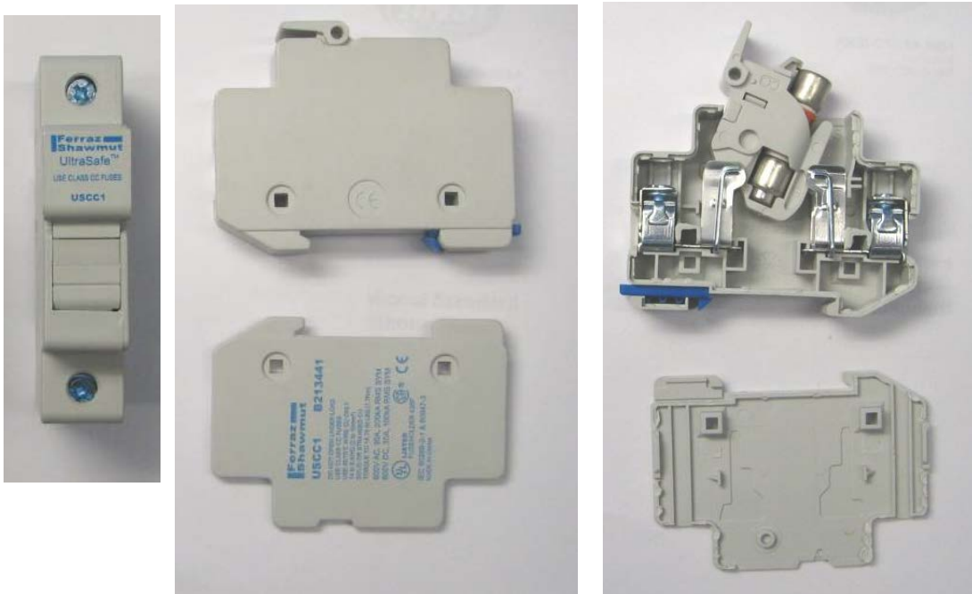
Figure 4.—A sample 10-A fuse: (Left) Front view, (Center) Exterior view of disassembled fuse, and (Right) Interior view of disassembled fuse
